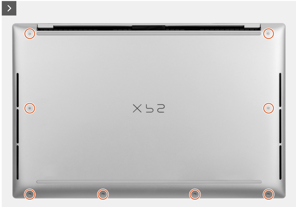
Figure 13. Removing the base cover
