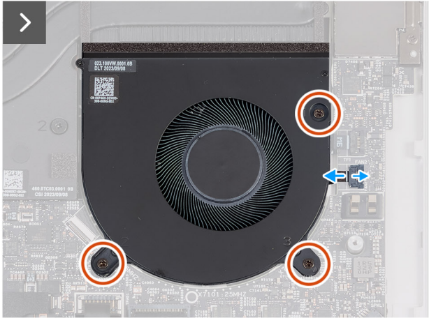
Figure 24. Removing the CPU fan
