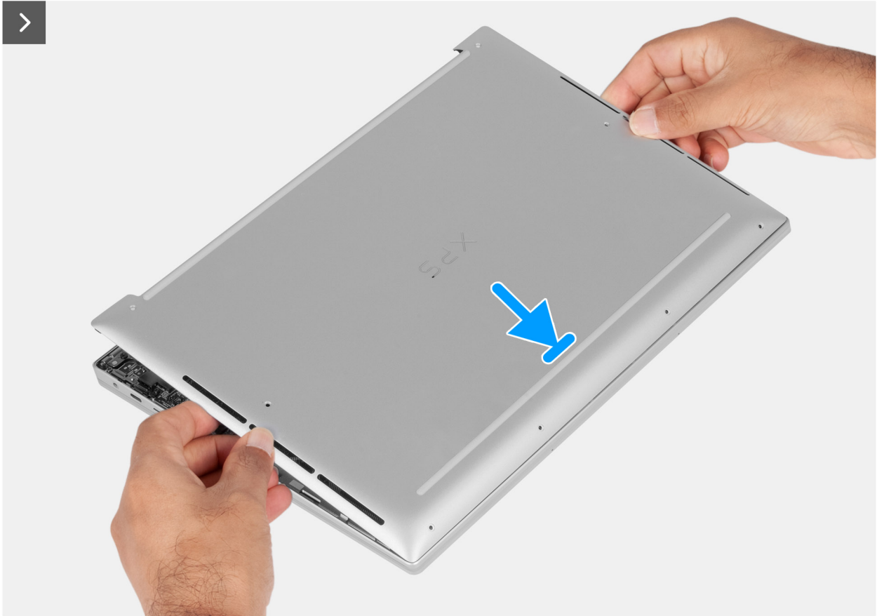
Figure 16. Installing the base cover
