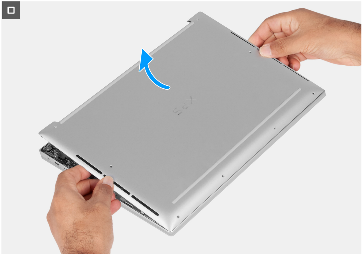
Figure 15. Removing the base cover
