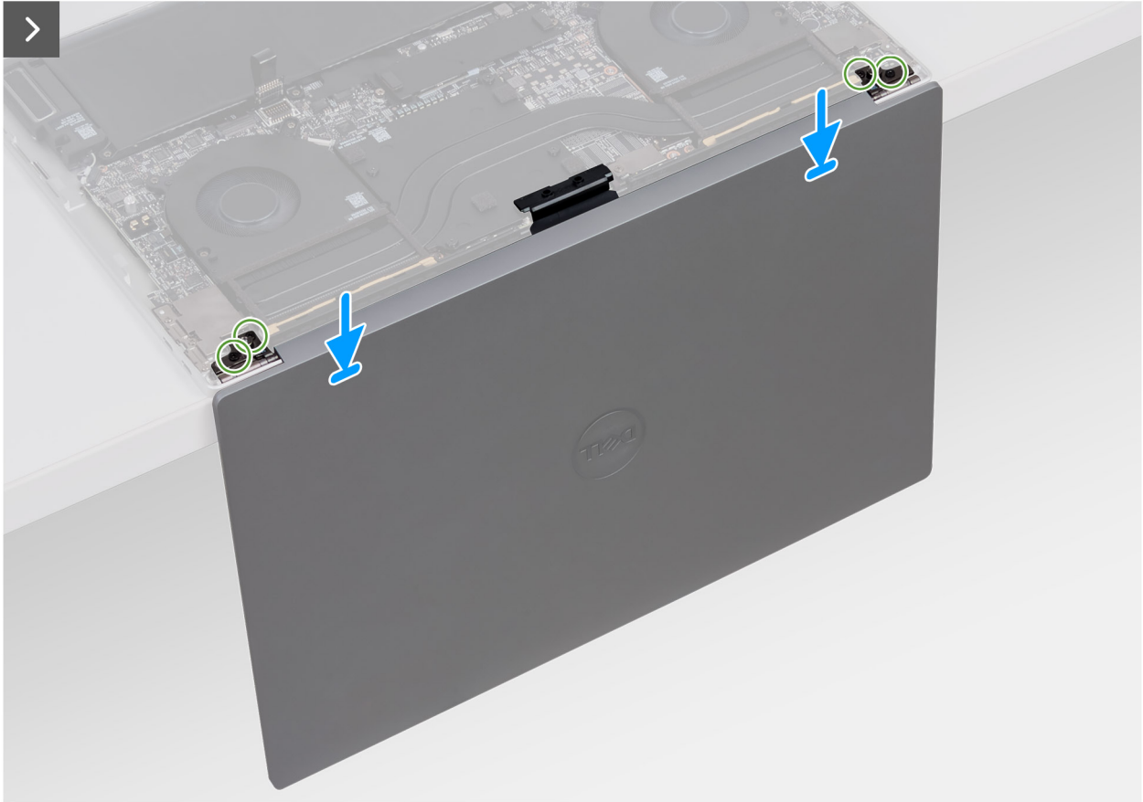
Figure 41. Installing the display assembly
