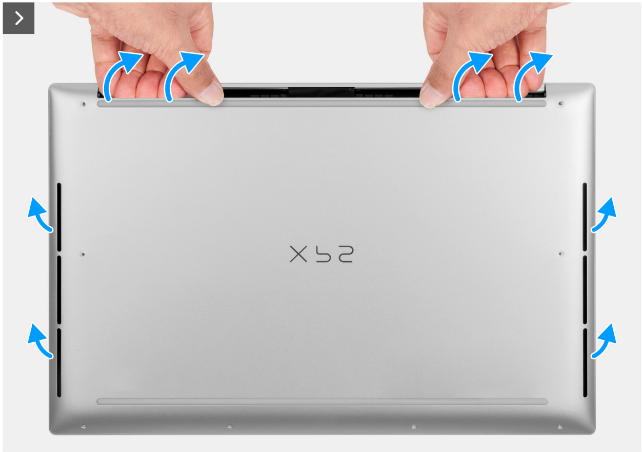
Figure 14. Removing the base cover
