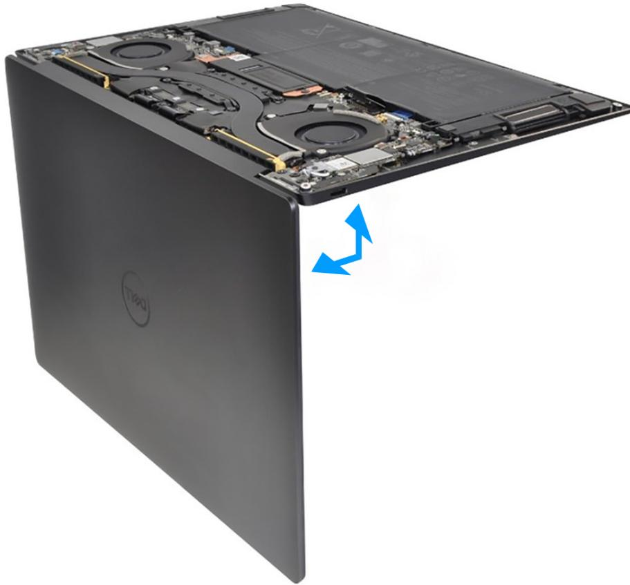
**Figure 53. Opening the display assembly to a 90-degree angle**
