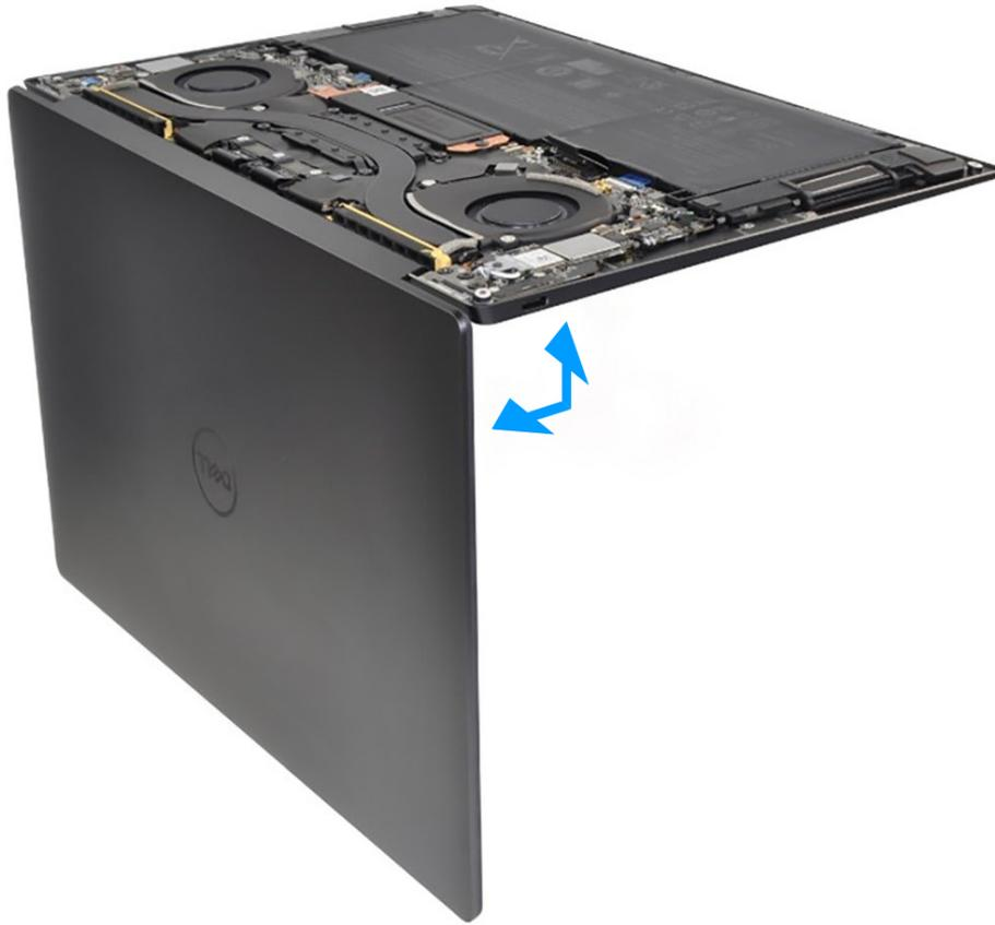
**Figure 47. Opening the display assembly to a 90-degree angle**
