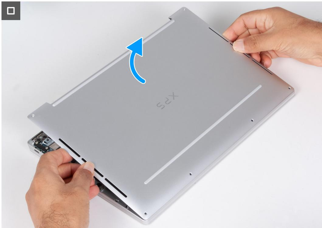
Figure 15. Removing the base cover
