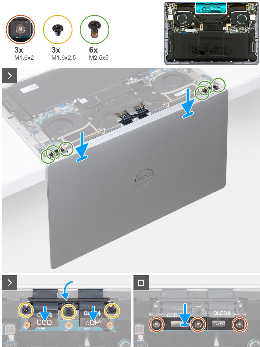
**Figure 35. Installing the display assembly**
