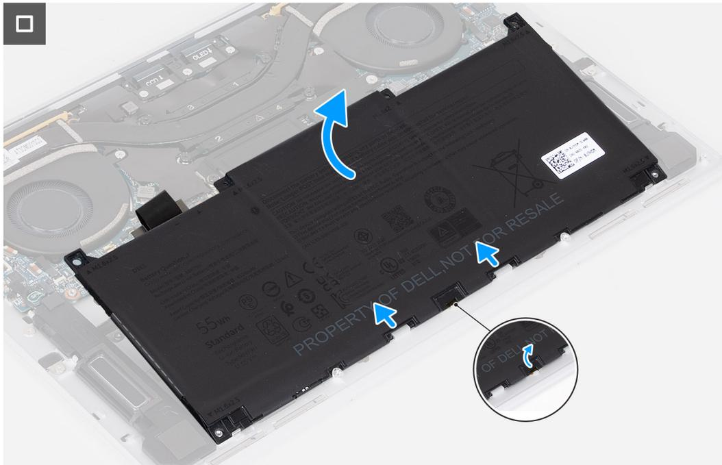
**Figure 19. Removing the battery**
