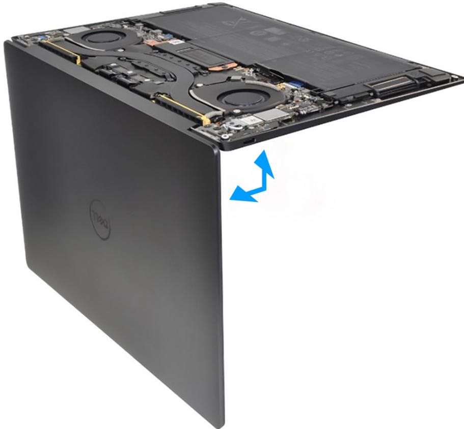
**Figure 43. Opening the display assembly to a 90-degree angle**
