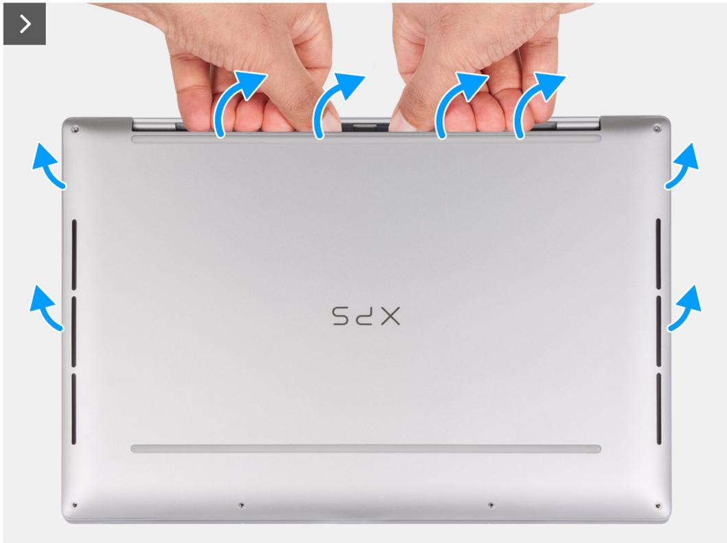
Figure 14. Removing the base cover
