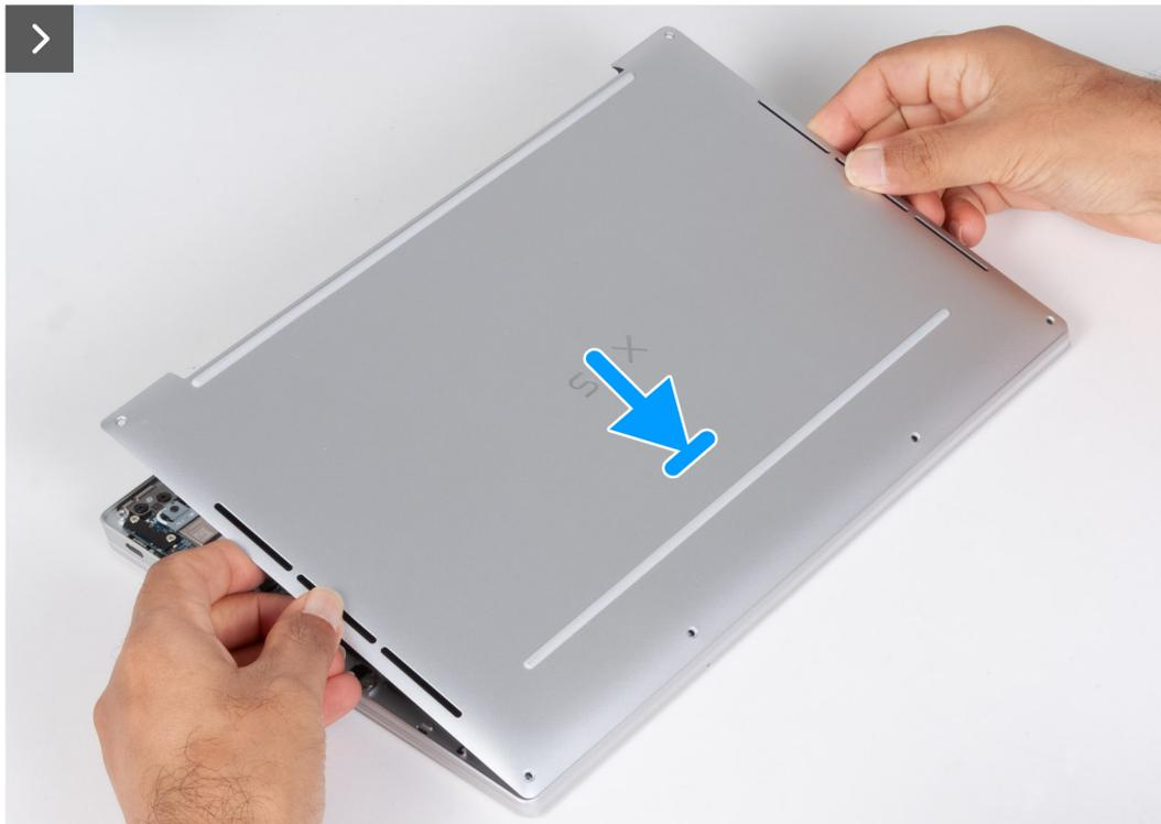
Figure 16. Installing the base cover
