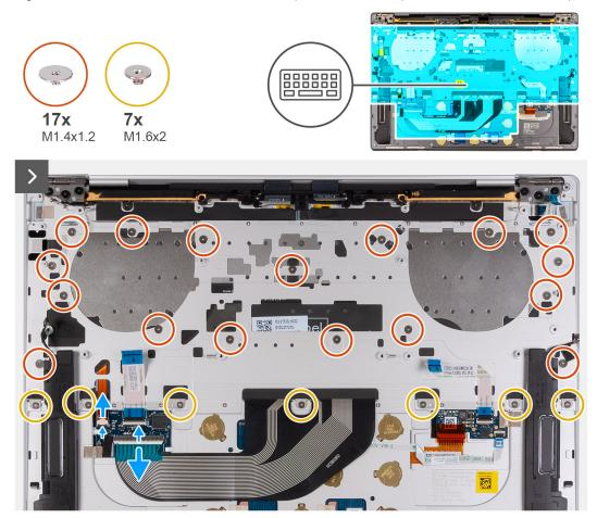
Figure 48. Removing the keyboard
