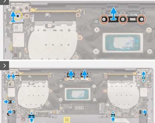
Figure 37. Removing the system board
