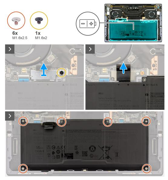
Figure 18. Removing the battery
