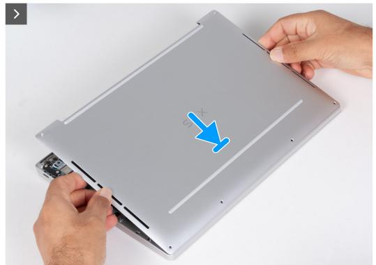
Figure 16. Installing the base cover
