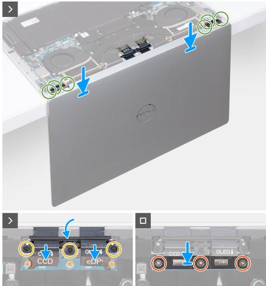
Figure 35. Installing the display assembly
