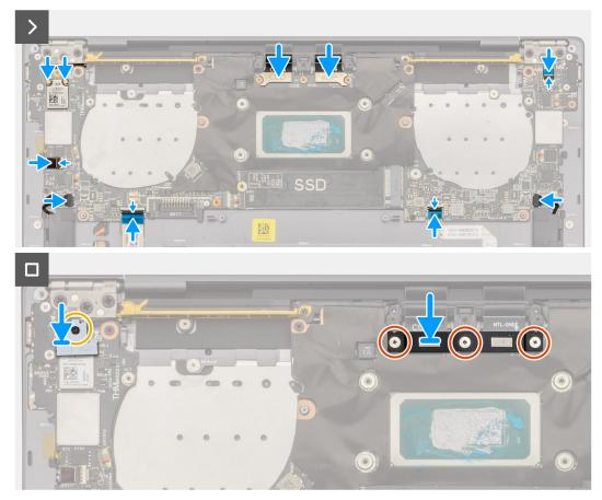
Figure 42. Installing the system board
