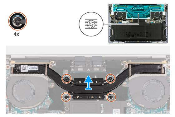
Figure 32. Removing the heat sink
