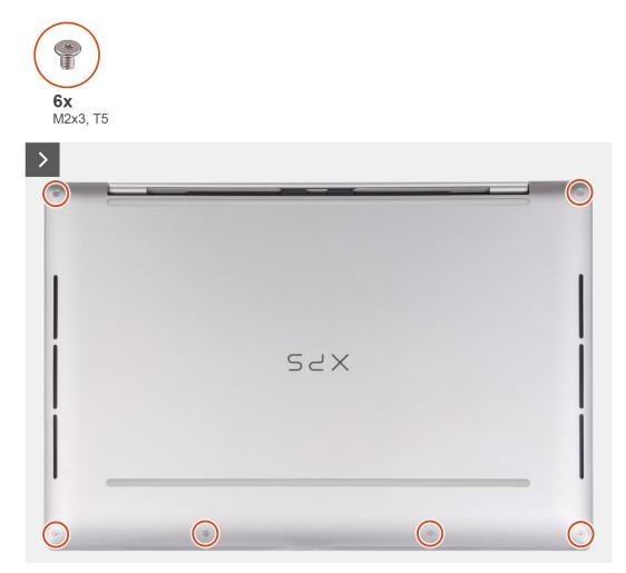
Figure 13. Removing the base cover
