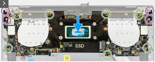
Figure 41. Installing the system board
