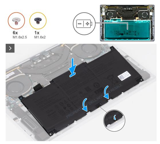
Figure 22. Installing the battery
