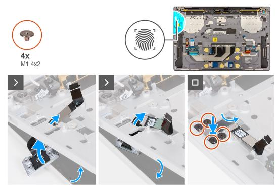
Figure 46. Installing the power button with fingerprint reader
