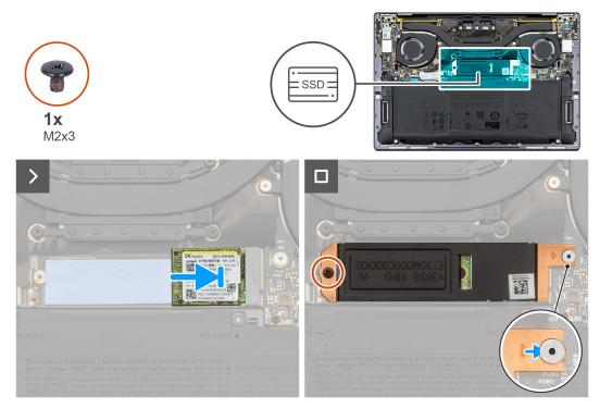
Figure 25. Installing the M.2 2230 solid-state drive
