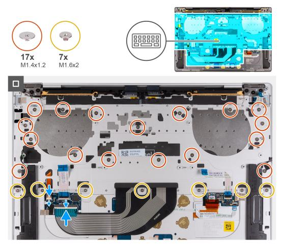
Figure 52. Installing the keyboard
