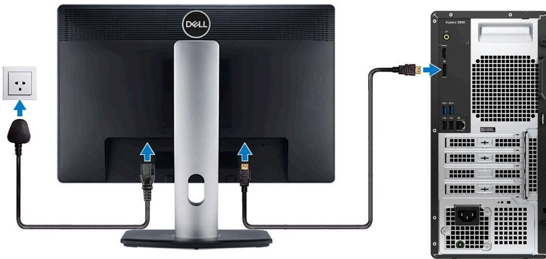
**i** **NOTE:** The location to connect the display cable can vary if your computer has a discrete graphics card installed. For optimal graphics performance, ensure to connect the display cable to the graphics card if there is one installed.
