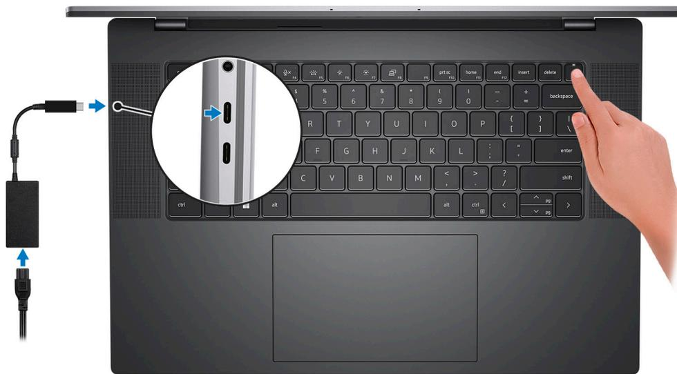
**NOTE:** To conserve battery power, the battery might enter power saving mode. Connect the power adapter and press the power button to turn on the computer.
