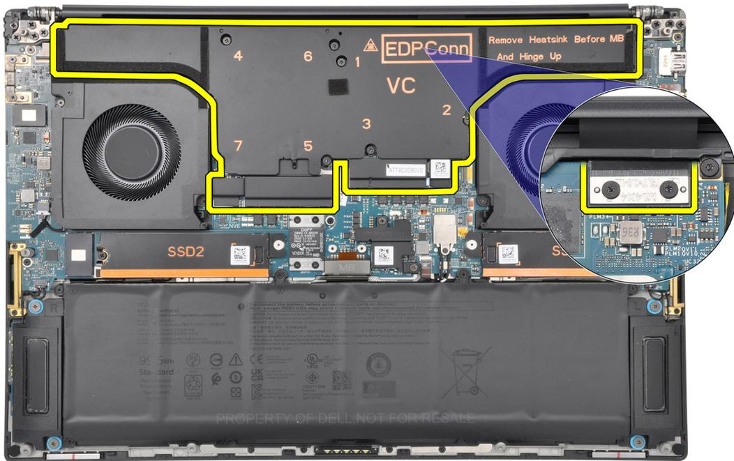
**NOTE:** Thermal pads (thermal conductors) are on the heatsink. If the heatsink is replaced, the new heatsink is shipped with thermal pads. Ensure all thermal pads are in place between the heatsink and the system board.
