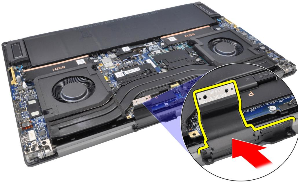
5. Replace the two (M1.4x4) T5 Torx screws to secure the display FPC cable in place.
