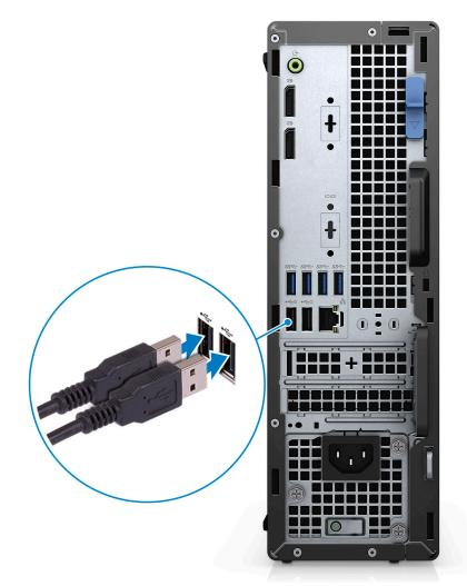
2. Connect to your network using a cable, or connect to a wireless network.
