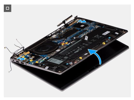
Figure 50. Removing the display assembly
