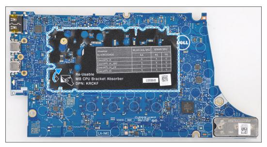
Figure 62. CPU bracket absorber
