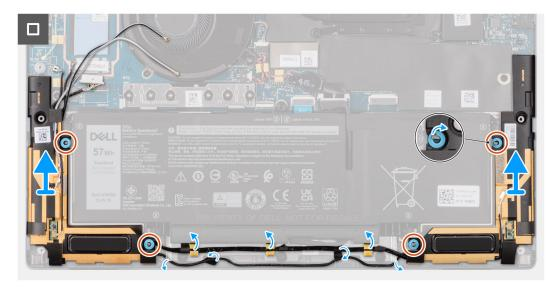
Figure 30. Removing the speakers for ultralight
