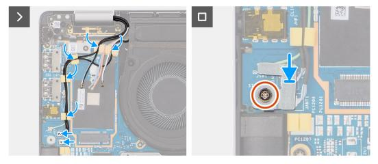
Figure 55. Installing the display assembly
