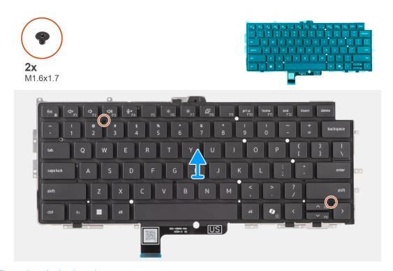
Figure 79. Removing the keyboard
