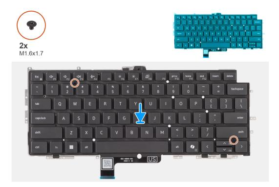
Figure 82. Installing the keyboard
