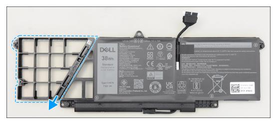
Figure 38. Removing the 2-cell battery
