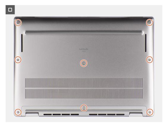
Figure 21. Installing the base cover
