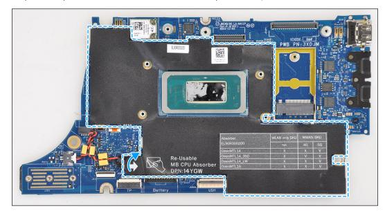
Figure 61. CPU absorber
