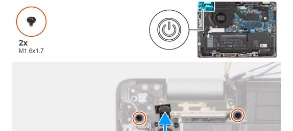
Figure 76. Removing the power button with optional fingerprint reader
