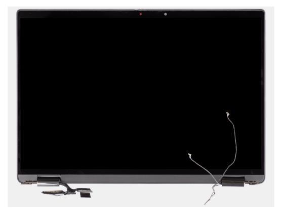
Figure 51. Display assembly with WWAN-antenna cables
