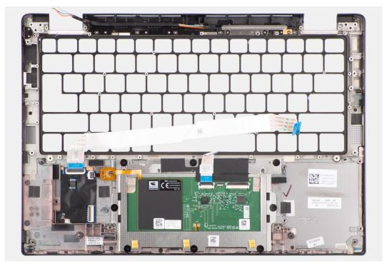
Figure 84. Removing the palm-rest assembly
