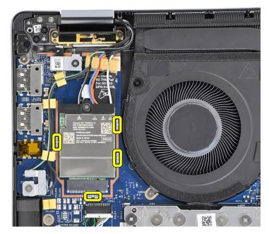
Figure 28. Installing the 5G WWAN card
