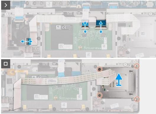
Figure 56. Removing the smart card reader
