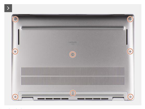
Figure 16. Removing the base cover
