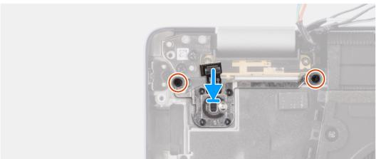
Figure 77. Installing the power button with optional fingerprint reader
