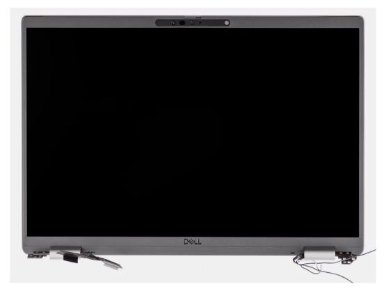
Figure 52. Display assembly with WWAN-antenna cables
