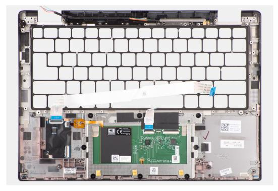
Figure 85. Installing the palm-rest assembly
