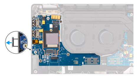
Figure 70. Removing the I/O daughterboard
