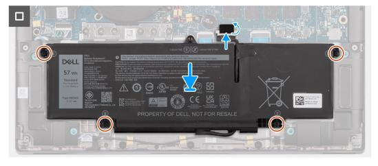
Figure 43. Installing the 3-cell battery
