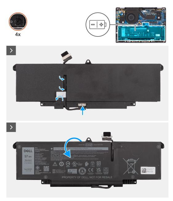
Figure 42. Installing the 3-cell battery
