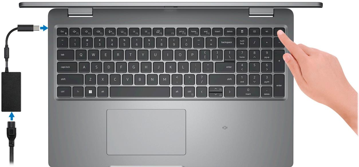
**NOTE:** To conserve battery power, the battery might enter power saving mode. Connect the power adapter and press the power button to turn on the computer.
