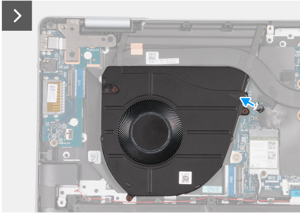
Figure 17. Removing the fan
