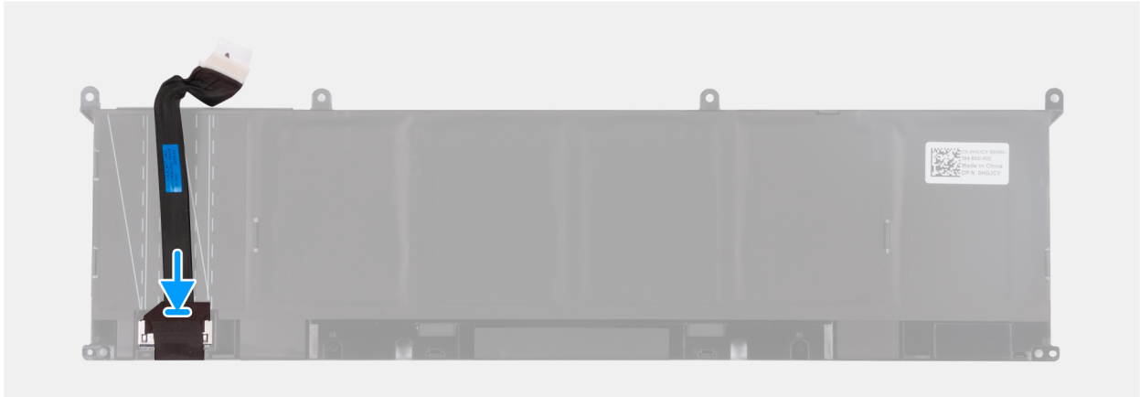
Figure 28. Installing the 90 Wh battery cable
