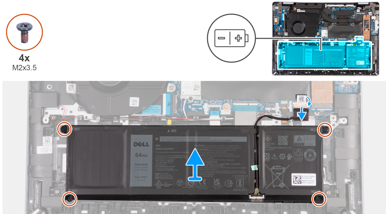
Figure 21. Removing the 4-cell battery (64 Wh)
