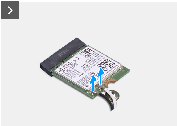
Figure 19. Removing the wireless card
