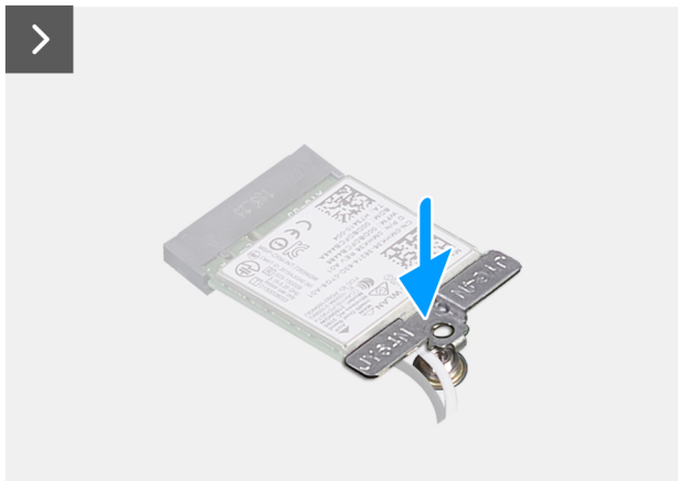
Figure 20. Installing the wireless card
