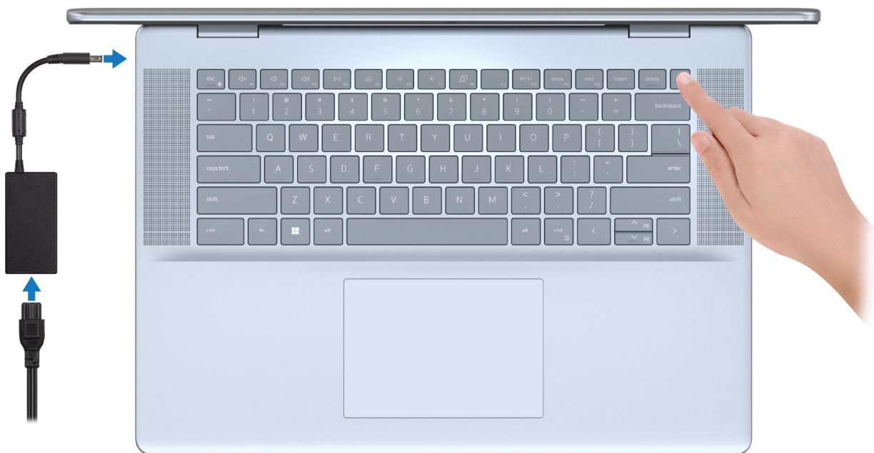
Figure 7. Connect the power adapter
