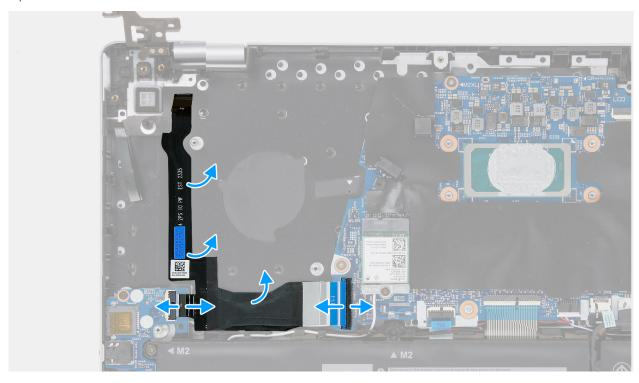
Figure 49. Removing the I/O-board and USB-board cable
