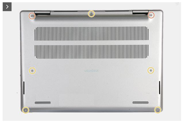
Figure 9. Removing the base cover
