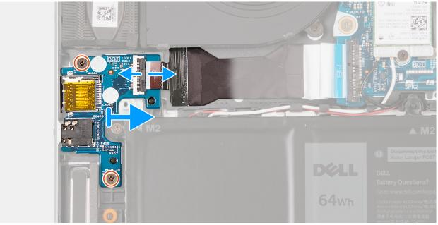
Figure 28. Removing the IO board
