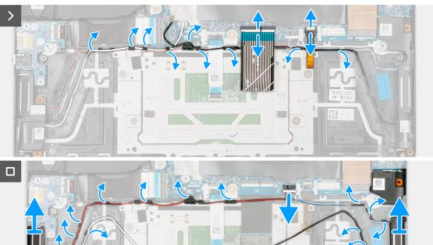
Figure 30. Removing the speaker and antenna assembly
