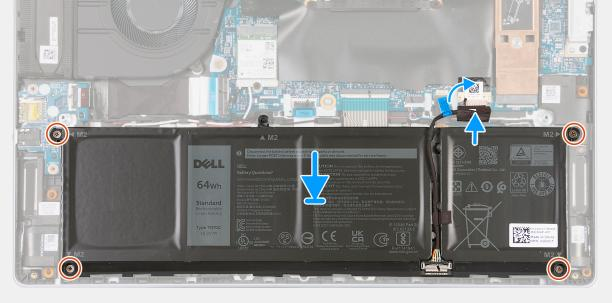
Figure 22. Installing the battery
