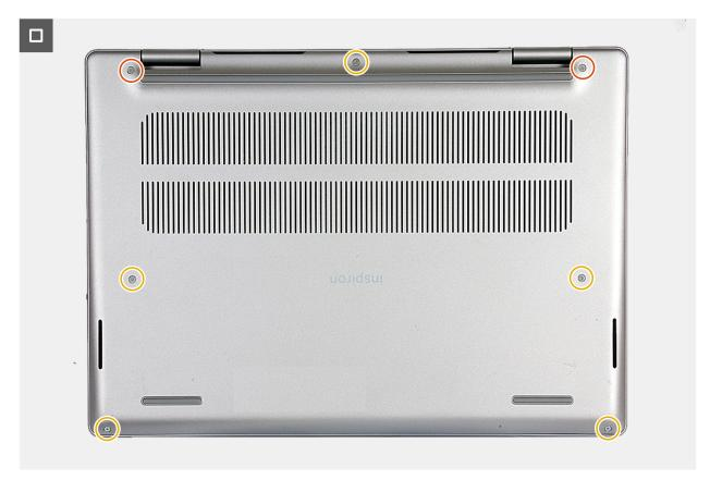
Figure 12. Installing the base cover 2
