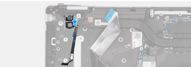
Figure 45. Installing the power button with an optional fingerprint reader
