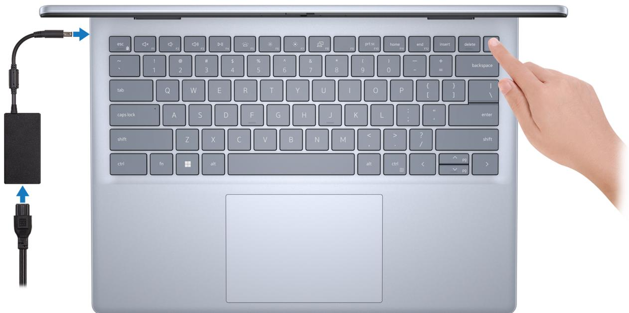
**Figure 7. Connect the power adapter**
