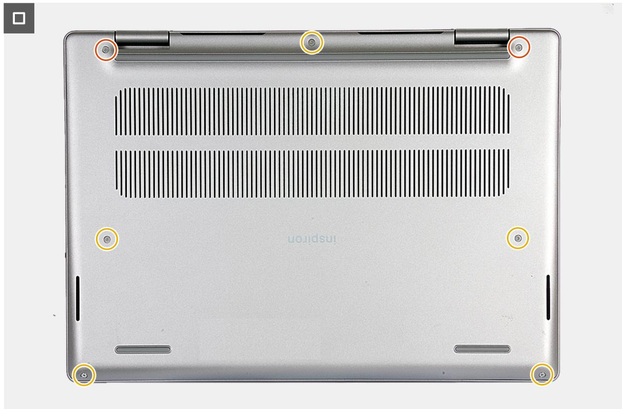
Figure 12. Installing the base cover 2
