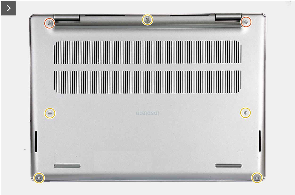
Figure 9. Removing the base cover
