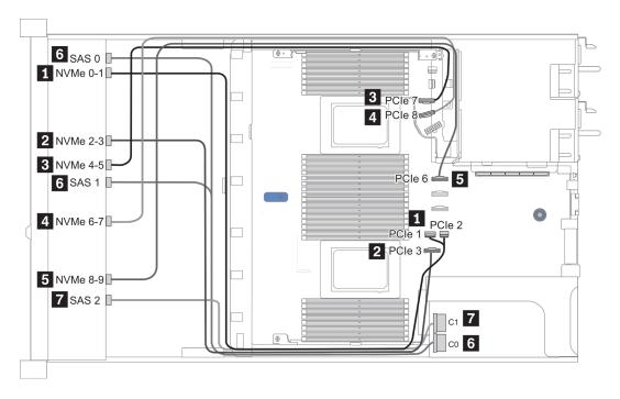
Figure 24. Cable routing for configuration 1
