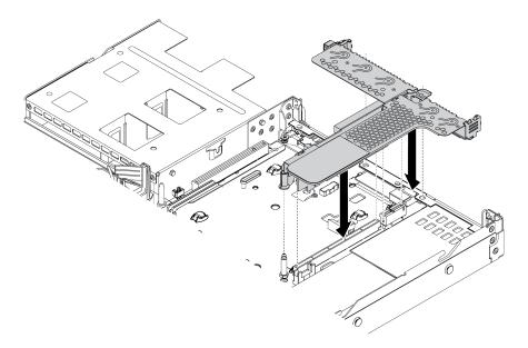
Figure 59. Riser assembly installation
