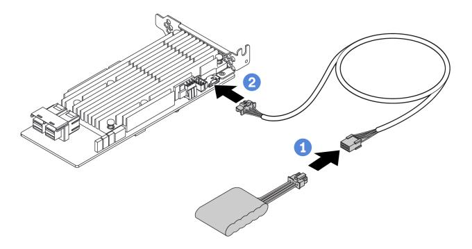
Figure 12. Power cable routing for super capacitor
