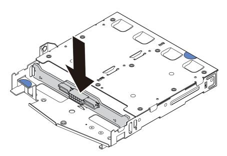
Figure 46. Rear backplane installation
