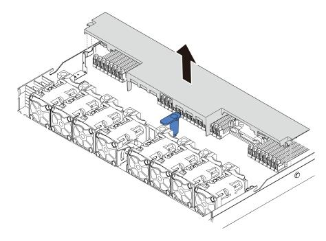
Figure 35. Air baffle removal
