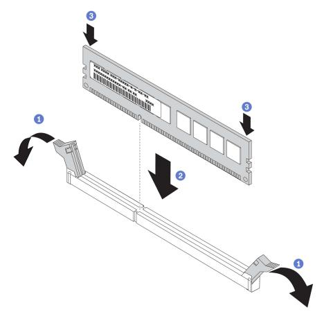
Figure 39. Memory module installation
