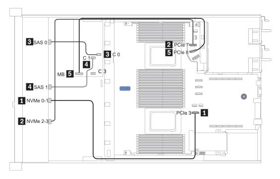
Figure 30. Cable routing for configuration 3
