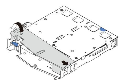
Figure 47. Air baffle installation
