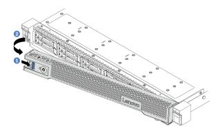
Figure 33. Security bezel removal
