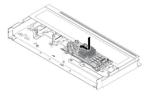
Figure 61. Internal RAID adapter installation
