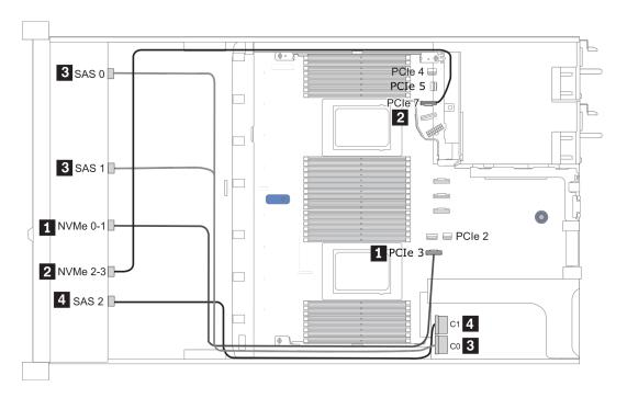
Figure 27. Cable routing for configuration 2
