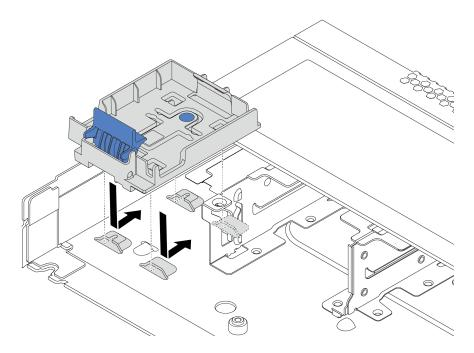
Figure 66. RAID super capacitor module holder installation
