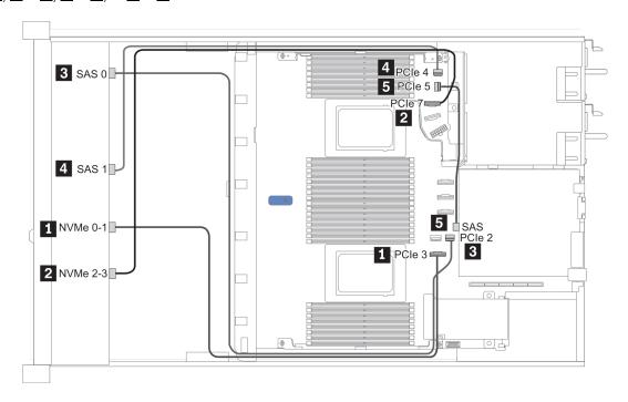
Figure 29. Cable routing for configuration 1
