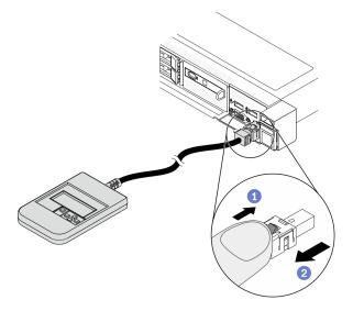
Step 1. Press the plastic clip on the plug in the shown direction.
