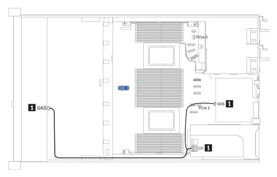
Figure 19. Cable routing for configuration 4
