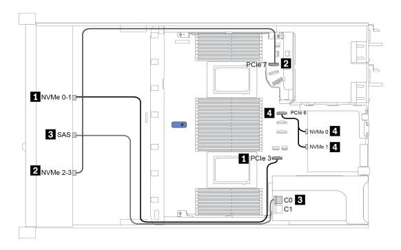
Figure 23. Cable routing for configuration 6
