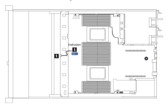
Figure 11. Intrusion switch cable routing
