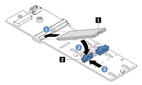
Figure 50. M.2 drive installation
