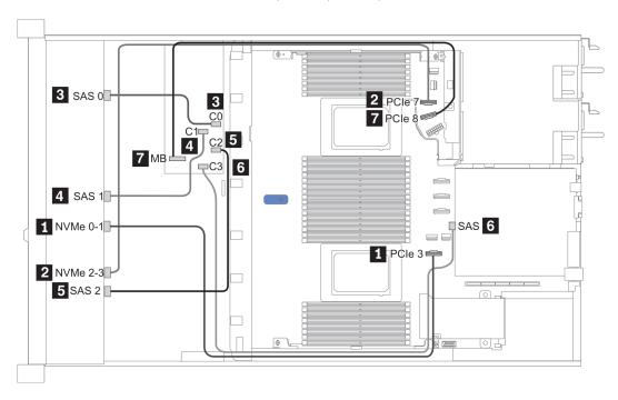
Figure 28. Cable routing for configuration 5
