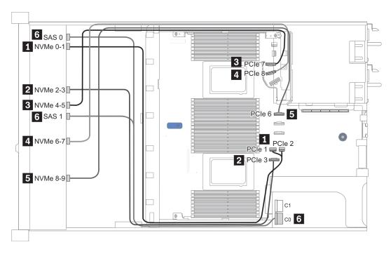
Figure 26. Cable routing for configuration 1
