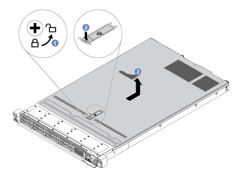
Figure 34. Top cover removal
