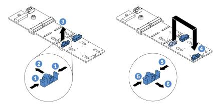
Figure 51. M.2 retainer adjustment
