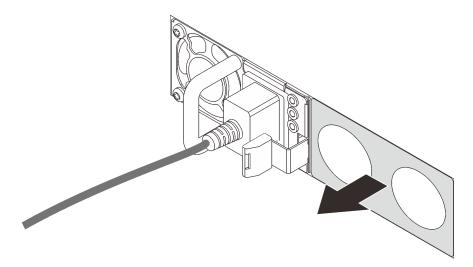
Figure 75. Hot-swap power supply filler removal
