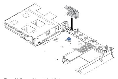
Figure 60. Rear wall bracket installation
