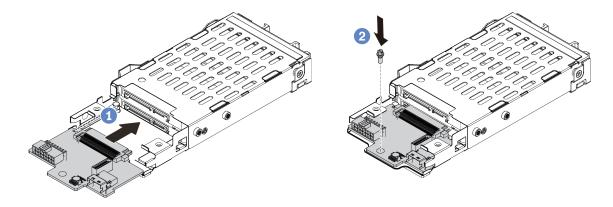
Figure 43. 7mm drive backplane installation (bottom)
