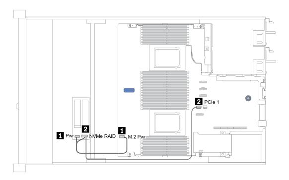
Figure 14. Cable routing for M.2 drives
