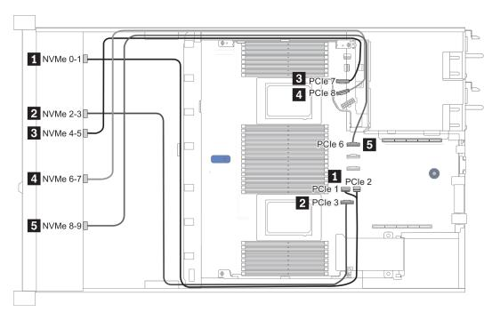
Figure 25. Cable routing for configuration 2
