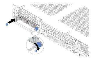
Figure 69. OCP 3.0 Ethernet adapter installation
