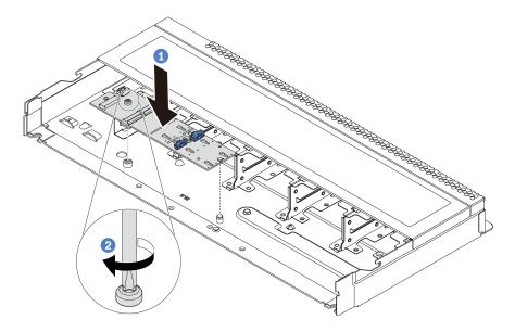
Figure 49. M.2 adapter installation
