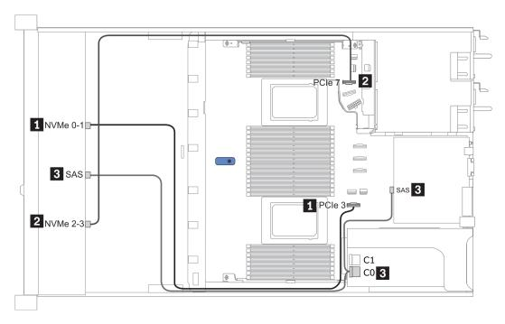
Figure 22. Cable routing for configuration 4
