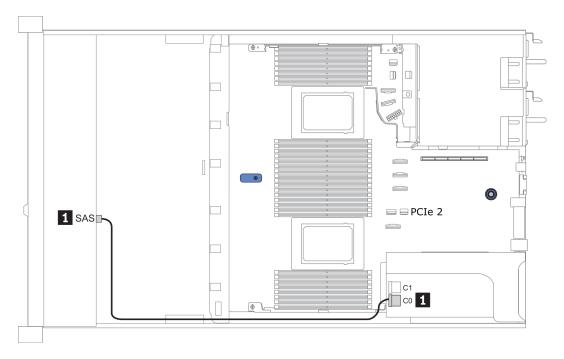
Figure 18. Cable routing for configuration 2
