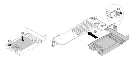
Figure 63. Installation of the RAID super capacitor module on the riser
