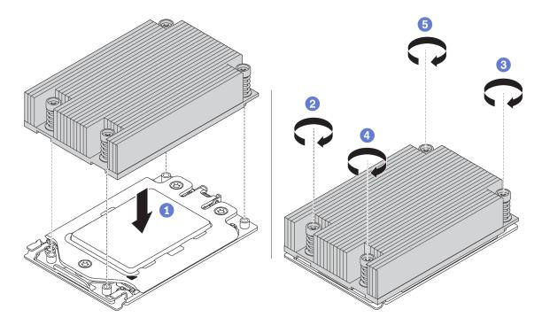
Figure 37. Standard heat sink installation
