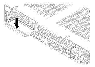
Figure 68. OCP 3.0 Ethernet adapter label installation
