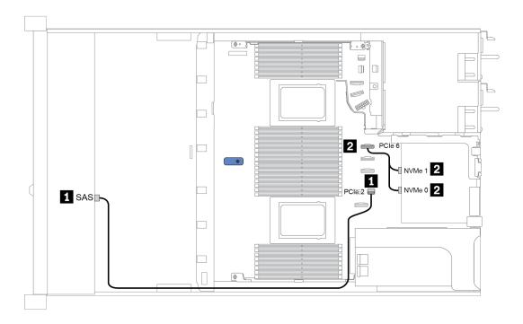
Figure 20. Cable routing for configuration 5
