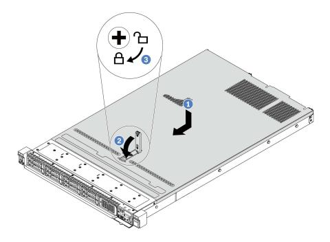
Figure 73. Top cover installation
