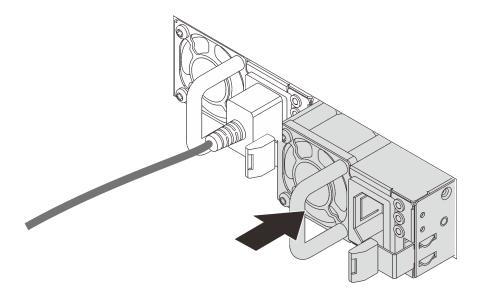
Figure 76. Hot-swap power supply installation
