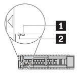
Figure 4. Drive LEDs
