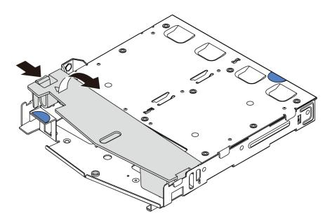
Figure 54. Air baffle removal
