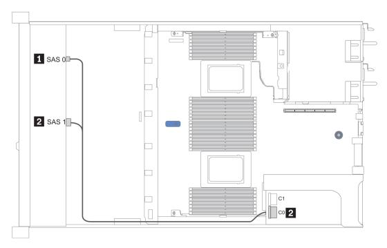
Figure 16. Cable routing for configuration 2
