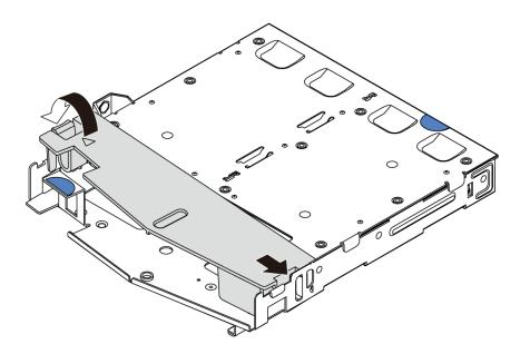
Figure 56. Air baffle installation
