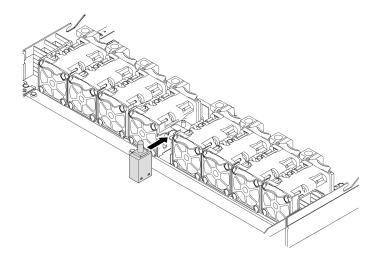
Figure 71. Intrusion switch installation
