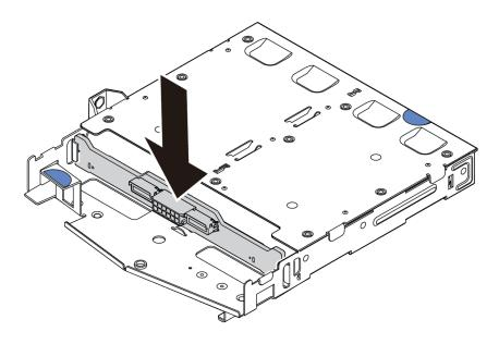
Figure 55. Rear backplane installation
