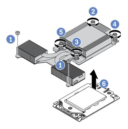
Figure 38. Performance heat sink installation
