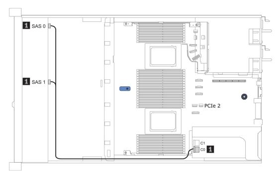
Figure 15. Cable routing for configuration 2
