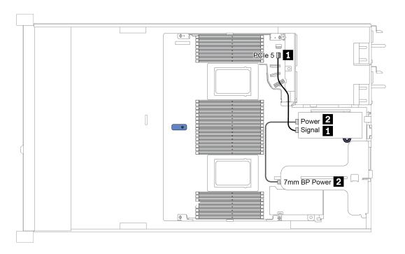
Figure 13. Cable routing for 7mm drives
