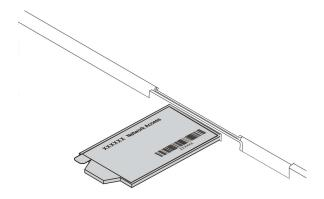
Figure 2. Location of the XClarity Controller network access label
