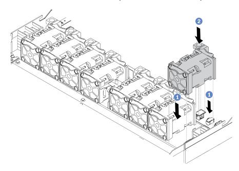
Figure 70. System fan installation
