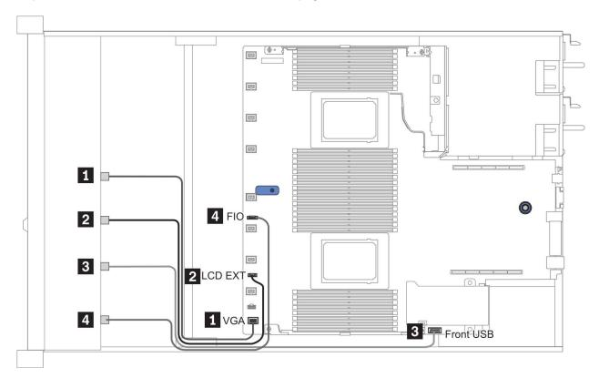
Figure 10. Cable routing for FIO
