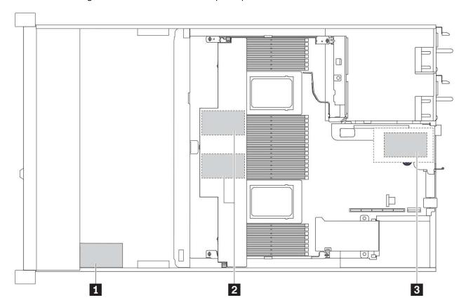
Figure 62. RAID super capacitor module location
