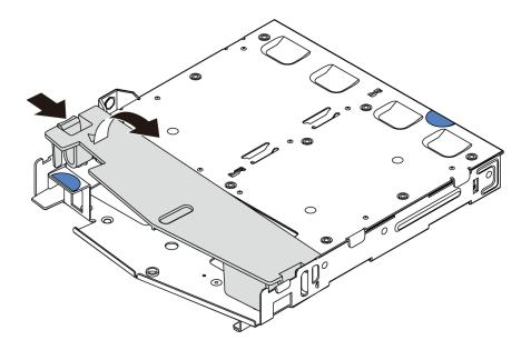
Figure 45. Air baffle removal
