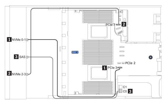
Figure 21. Cable routing for configuration 2
