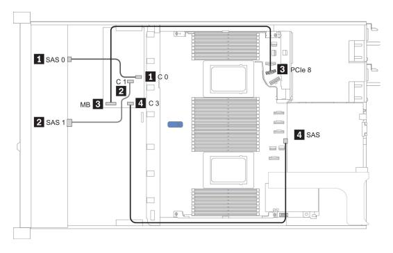
Figure 17. Cable routing for configuration 6
