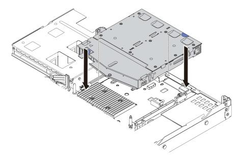
Figure 57. Rear hot-swap drive cage installation
