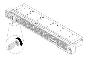
Figure 32. Unlocking the security bezel
