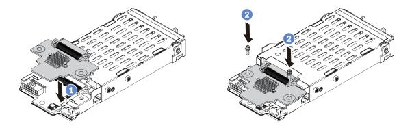
Figure 44. 7mm drive backplane installation (top)
