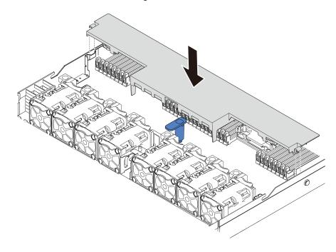
Figure 72. Air baffle installation
