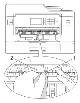
7. Put the paper support firmly back in the machine. Make sure you fit the paper support into the channels.
