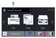
[Stored Faxes] displays how many received faxes are in the machine's memory.
