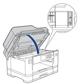
• If the paper is jammed under the print head, unplug the machine from the power source, and then move the print head to take out the paper.
