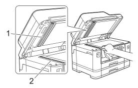
4. (MFC-J2730DW/MFC-J5730DW/MFC-J5930DW) Open the scanner glass cover (1), and clean the white bar (2) and the glass strip (3) with a soft lint-free cloth moistened with water.
