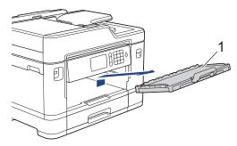
5. Clean the front side of the Paper Feed Rollers (1) with a soft lint-free cloth moistened with water, using a side-to-side motion. After cleaning, wipe the rollers with a dry, soft lint-free cloth to remove all moisture.
