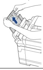
2. Gently press and slide the MP tray paper guides to match the width of the paper you are using.
