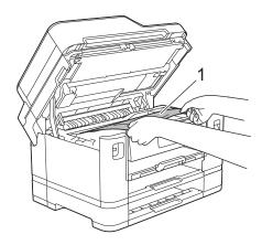
If your LCD error message was repeat paper jam messages, for example [Repeat Jam Rear], move the print head (if necessary) to take out any paper remaining in this area. Make sure pieces of paper are not left in the corners of the machine (1) and (2).
