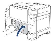
5. If your LCD error message was [Jam MP Tray] or [Repeat Jam MP Tray], push the release lever (1) towards the back of the machine, and then slowly pull the jammed paper out of the MP tray.
