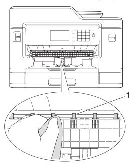
6. Lift the Jam Clear Flap (2), and then clean the back side of the Paper Feed Rollers (1) with a soft lint-free cloth moistened with water. After cleaning, wipe the rollers with a dry, soft lint-free cloth to remove all moisture.
