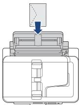
When loading an envelope, or a sheet of thick paper, push the envelope into the manual feed slot until
