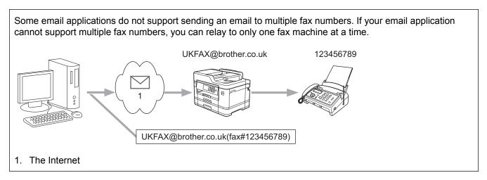
If you are sending an email to a conventional fax machine, the method of entering the fax machine's fax number will vary, depending on the mail application you are using.
