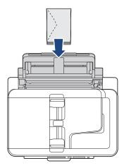
If you are having difficulty loading paper in the MP tray, push the release lever (1) towards the back of the machine, and then load the paper.
