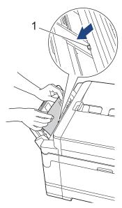
6. If your LCD error message was [Jam Manual Feed Slot] or [Repeat Jam Manual Feed Slot], slowly pull the jammed paper out of the manual feed slot.
