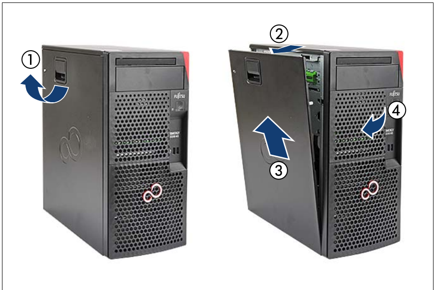
Figure 4: Removing the side cover
