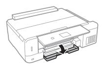
4. Check that the printer is not operating, and then pull out paper cassette 1. Paper cassette 1 has an alignment mark that allows you to locate it easily.
