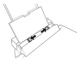
4. Load paper at the center of the rear paper feed with the printable side facing up.
