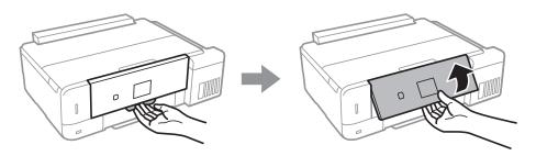
2. When the output tray is ejected, check that there is no paper on the tray, and then close it by pushing it with your hand.
