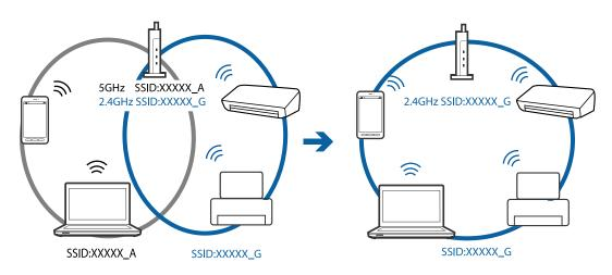
□ Most access points have a privacy separator feature that blocks communication between connected devices. If you cannot communicate between the printer and the computer or smart device even if they are connected to the same network, disable the privacy separator on the access point. See the manual provided with the access point for details.
