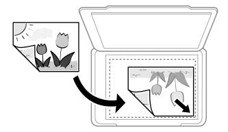
*Note: A range of 1.5 mm from the edges of the scanner glass is not scanned.*
