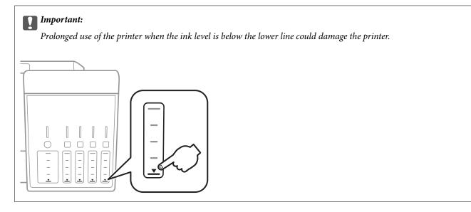
You can check the approximate ink levels from the computer, and the approximate service life of the maintenance box from the control panel or the computer.
