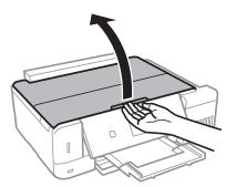
2. Use a soft, dry, clean cloth to clean the surface of the scanner glass.
