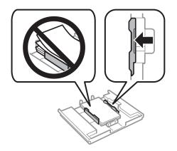
9. Insert paper cassette 1. Line up the alignment marks on the printer and the tray.
