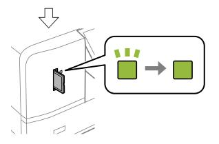
2. When you have finished using the memory card, make sure the light is not flashing, and then remove the card.
