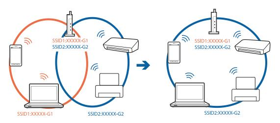
□ An access point that is compliant with both IEEE802.11a and IEEE802.11g has SSIDs of 2.4 GHz and 5 GHz. If you connect the computer or smart device to a 5 GHz SSID, you cannot connect to the printer because the printer only supports communication over 2.4 GHz. Connect the computer or smart device to the same SSID as the printer.
