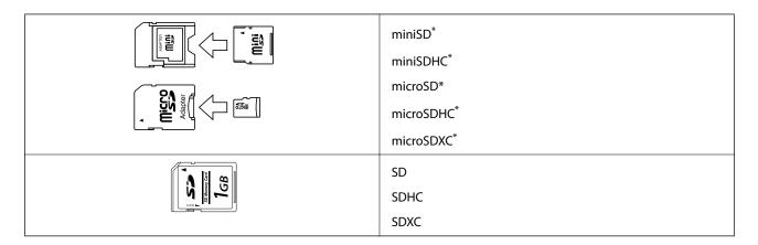
\* Attach an adapter to fit the memory card slot. Otherwise, the card may get stuck.
