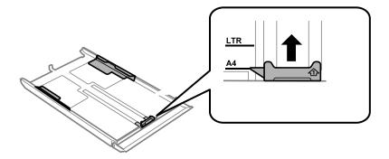
7. With the printable side facing down, load paper against the front edge guide.
