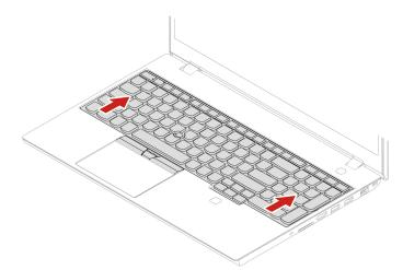
3. Pivot the keyboard slightly upward as shown by arrow **1** and then turn over the keyboard **2**.
