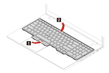
4. Put the keyboard on the palm rest as shown and detach the connectors. Then, remove the keyboard.
