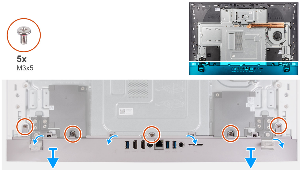
Figure 23. Removing I/O cover
