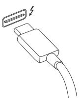
reversable; connectors may be inserted with either side up.
