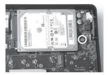
\*1TB hard disk drive is pre-installed in Plus and Windows version.
