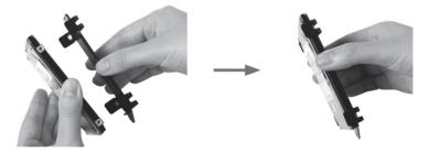
3. Insert the storage drive into the slot at a 45 degree angle and gently slide into the connector.
