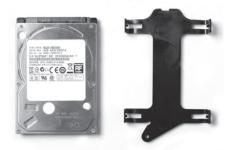
2. Install the storage drive to the storage drive bracket.
