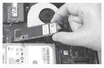
2. Gently press down on the M.2 SSD module, and install the screw.
