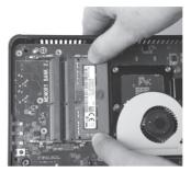
2. Remove the memory module from the slot at a 45-degree angle.
