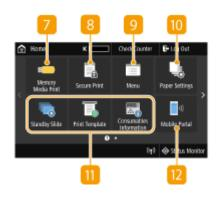
Displays the amount remaining in the toner cartridges in stages. This is hidden while the Home screen is active.
