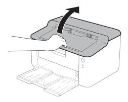
4 Slowly take out the drum unit and toner cartridge assembly. The jammed paper may be pulled out with the drum unit and toner cartridge assembly, or this may release the paper so you can pull it out from inside of the machine.
