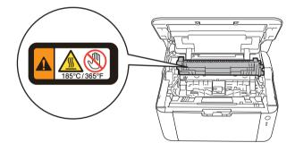
5 Push down the lock lever and take the toner cartridge out of the drum unit. Remove the jammed paper if there is any inside the drum unit.
