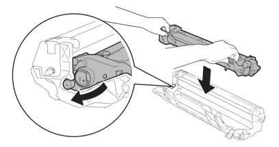
Put the drum unit and toner cartridge assembly back into the machine.
