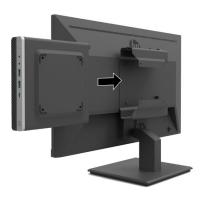
3. Install the DT Mini PC to the Dual VESA Sleeve V2.
