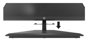
2. Insert the HP Speaker Bar into the speaker hole in the bottom of the monitor (1) and slide the HP Speaker Bar to the right (2).
