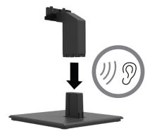
3. Insert the two tabs on the stand into the bracket on the back of the monitor head. You will hear a click when they are locked in place.
