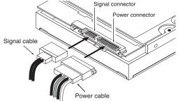
Each cable is keyed to ensure correct orientation. BarraCuda drives support latching SATA connectors.
