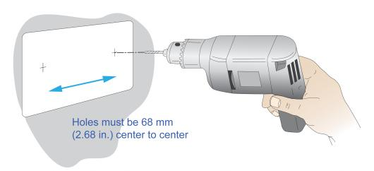
2. Install wall anchors in the holes.
