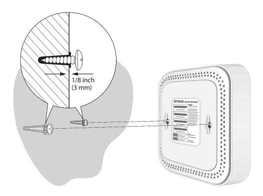
5. Attach the modem to the screws and secure it into place.
