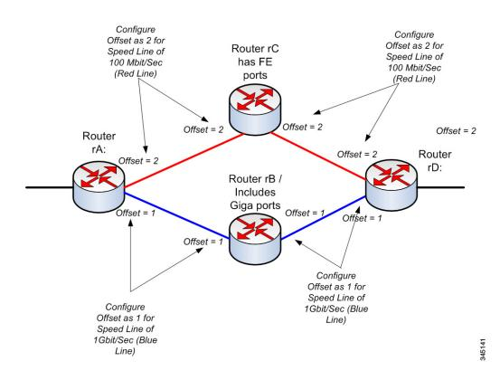
Router rD can send data to rA via rB or rC. Since rC only supports Fast Ethernet (FE) ports, and rB supports Gigabit Ethernet (GE) ports, the path cost from router rD to router rA is higher via router rC (additional 4 to the cost path) as opposed to the path via router rB (additional 2 to the cost path), Therefore, forwarding traffic via routing rB is preferred. To achieve this, you configure a different offset (metric value) on each interface based on its line speed.
