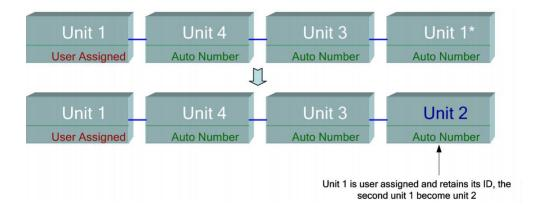
The following shows a case where one of the duplicate units is renumbered. The one with the lower MAC retains its unit ID (see Master Selection Process for a description of this process).
