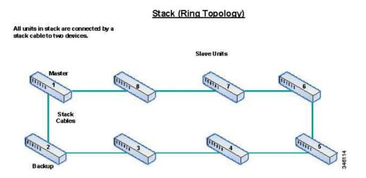
A ring topology is more reliable than a chain topology. The failure of one link in a ring does not affect the function of the stack, whereas the failure of one link in a chain connection might cause the stack to be split.
