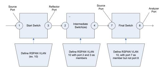
The traffic for each RSPAN session is carried over a user-specified RSPAN VLAN that is dedicated for that RSPAN session in all participating switches. The traffic from the source interfaces on the start device is copied to the RSPAN VLAN through a reflector port and then forwarded over trunk ports on the intermediate devices to the destination session on the final switch, which is monitoring the RSPAN VLAN.
