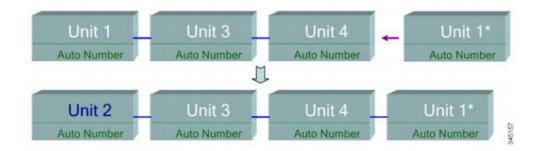
The following shows what happens when a user-assigned, master-enabled unit with Unit ID 1 joins a stack that already has a master unit with user-assigned unit ID 1. The newer Unit 1 does not join the stack and is shutdown.
