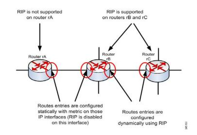
Router rA does not support RIP. Therefore, routing entries with an appropriate metric are configured statically on this router. While on router rB the route to router rA is considered a connected route. In contrast, routers rB and rC derive and distribute their routing entries using RIP.
