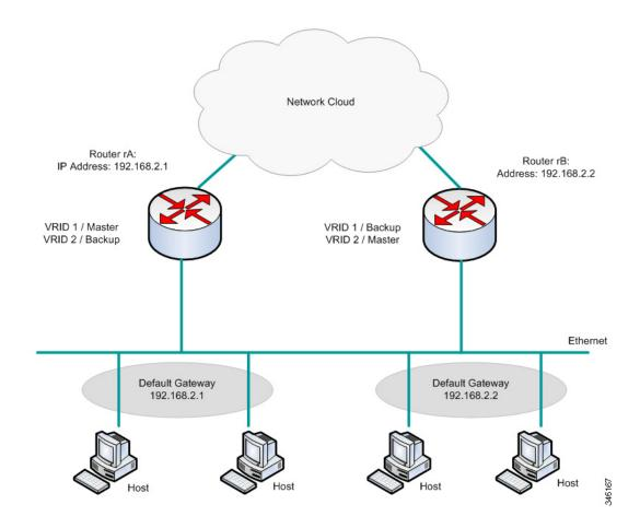
In this topology, two virtual routers are configured. For virtual router 1, rA is the owner of IP address 192.168.2.1 and is the virtual router master, and rB is the virtual router backup to rA. Clients 1 and 2 are configured with the default gateway IP address of 192.168.2.1.
