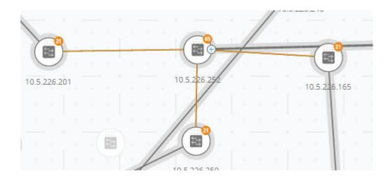
For example, in the below figure, the yellow lines show asymmetric connections, meaning where one end of the link is a member in the selected VLAN and the other end is not.
