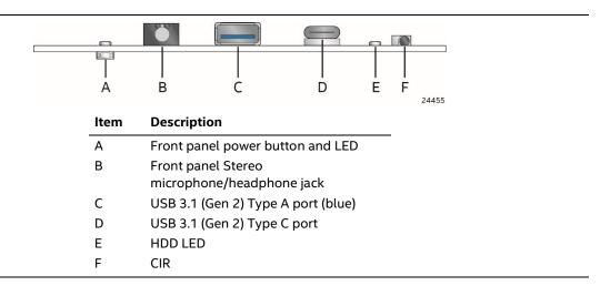
Figure 9. Front Panel Connectors
