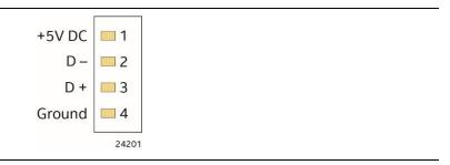
Figure 14. Connection Diagram for the Internal USB 2.0 Single-Port Header (1.25 mm Pitch)
