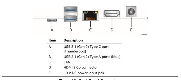
Figure 10. Back Panel Connectors
