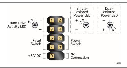
Figure 13. Connection Diagram for Front Panel Header (2.0 mm Pitch)
