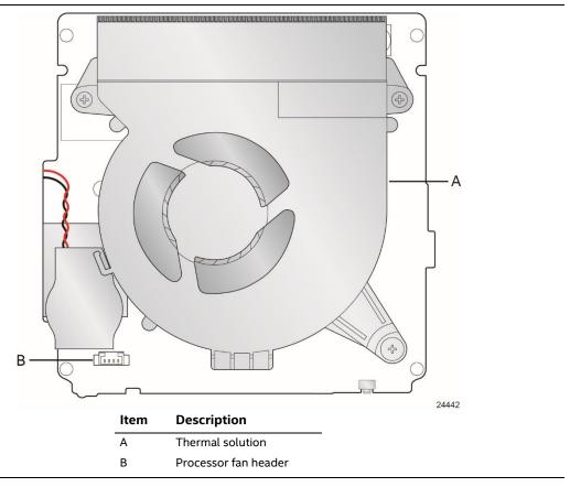
Figure 7. Thermal Solution and Fan Header
