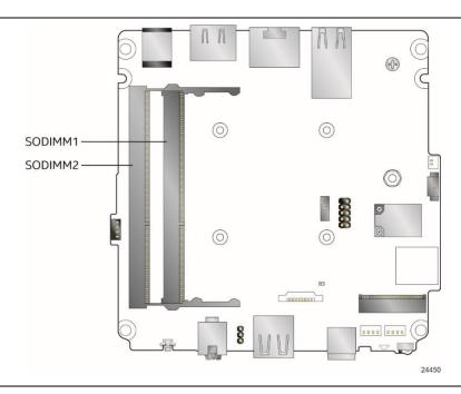
Figure 4. Memory Channel and SO-DIMM Configuration
