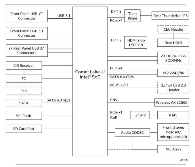
Figure 3. Block Diagram
