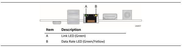
Figure 6. LAN Connector LED Locations
