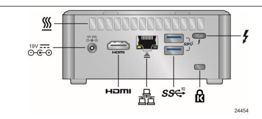
Figure 24. Intel NUC Kit NUC10i3FNH/NUC10i5FNH/NUC10i7FNH Features - Rear
