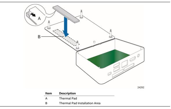
Figure 20. Installation Area of Thermal Pad for Intel NUC Kits NUC10i3FNK/NUC10i5FNK/NUC10i7FNK
