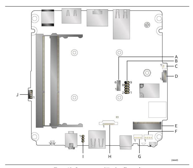
Figure 12. Connectors and Headers (Bottom)
