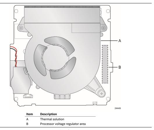
Figure 19. Localized High Temperature Zones
