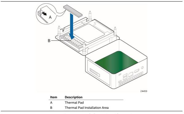
Figure 21. Installation area of Thermal Pad for Intel NUC Kits NUC10i3FNH/NUC10i5FNH/NUC10i7FNH
