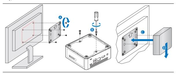
Figure 26. VESA Bracket Installation
