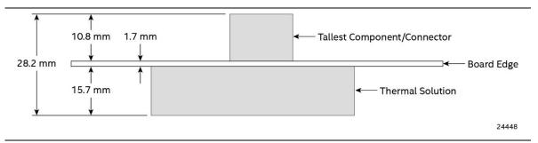
Figure 18. Board Height Dimensions
