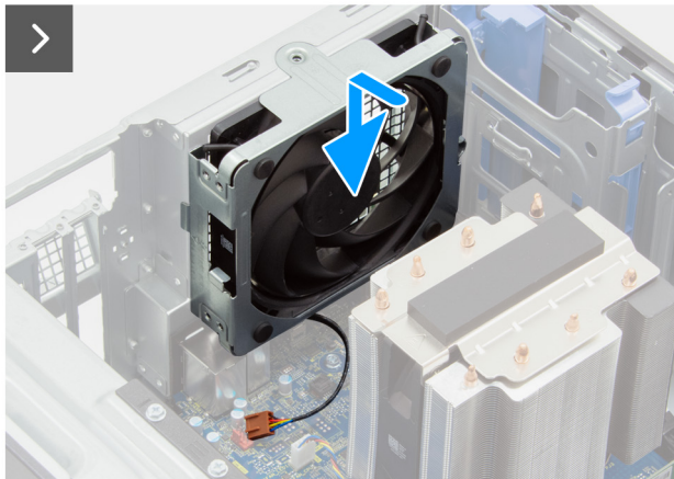
Figure 33. Installing the rear-chassis fan
