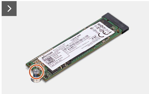
Figure 38. Removing the M.2 2280 solid-state drive
