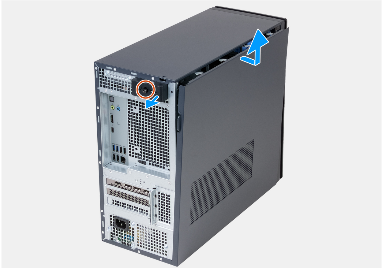
Figure 10. Removing the left-side cover
