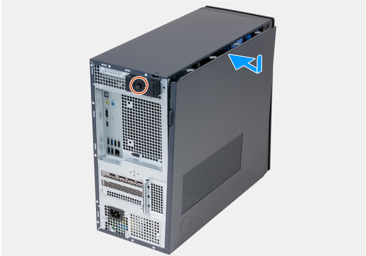
Figure 11. Installing the left-side cover
