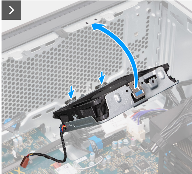
Figure 35. Installing the chassis fan
