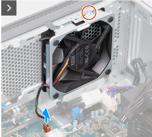
Figure 34. Removing the chassis fan
