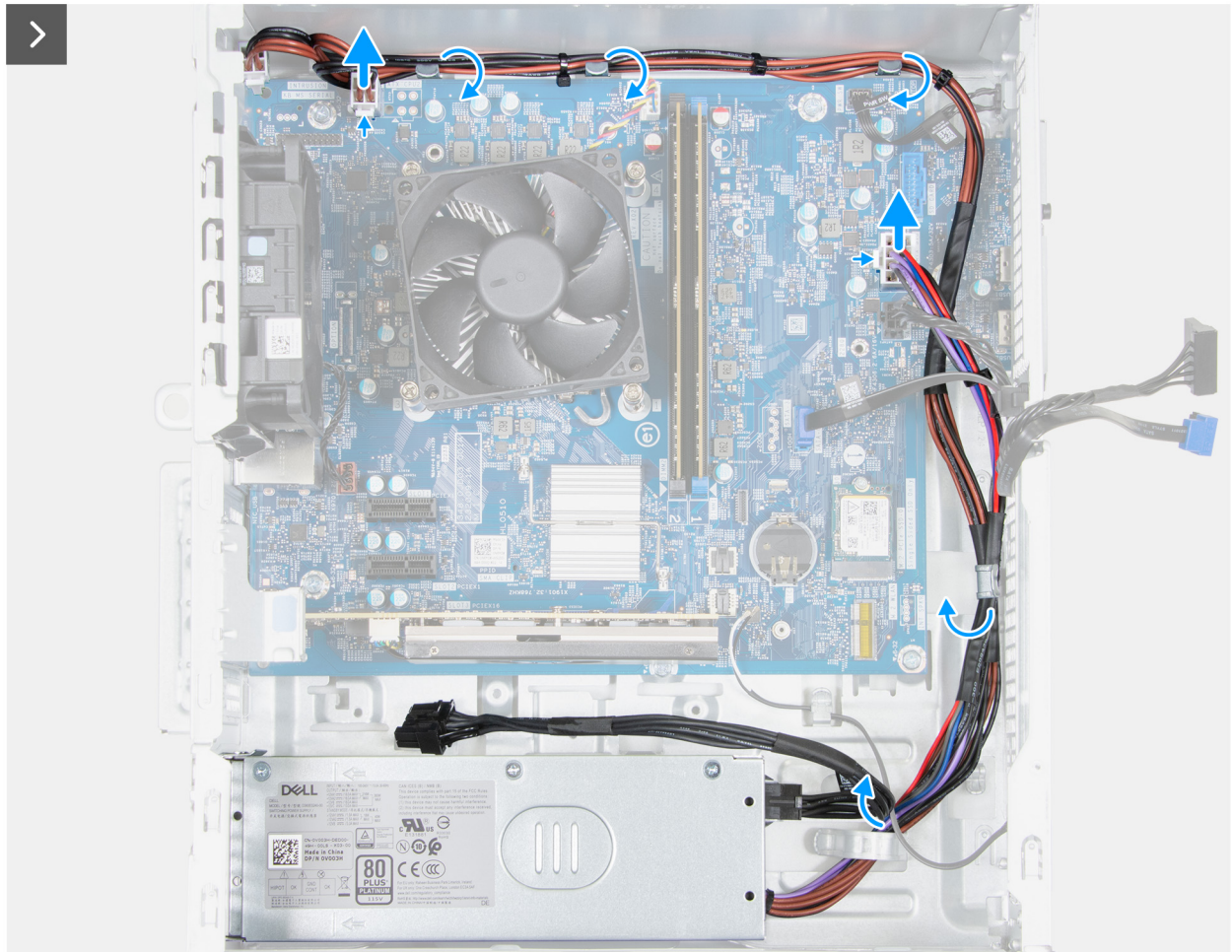
Figure 45. Removing the power-supply unit
