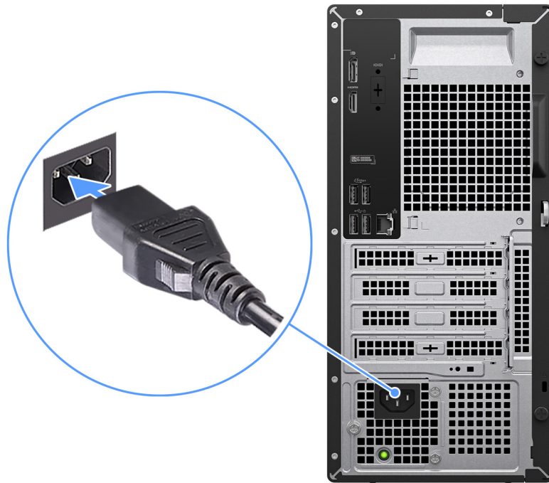
Figure 7. Connecting the power cable
