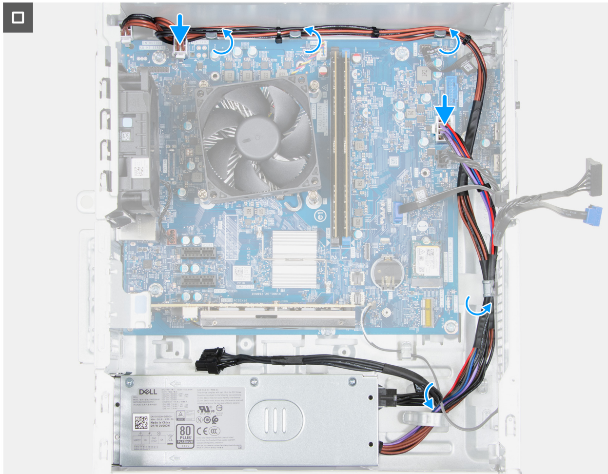
Figure 48. Installing the power-supply unit
