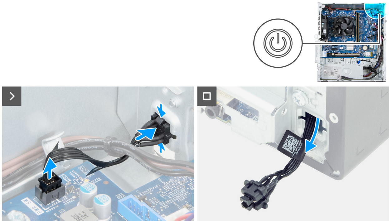
Figure 34. Removing the power button
