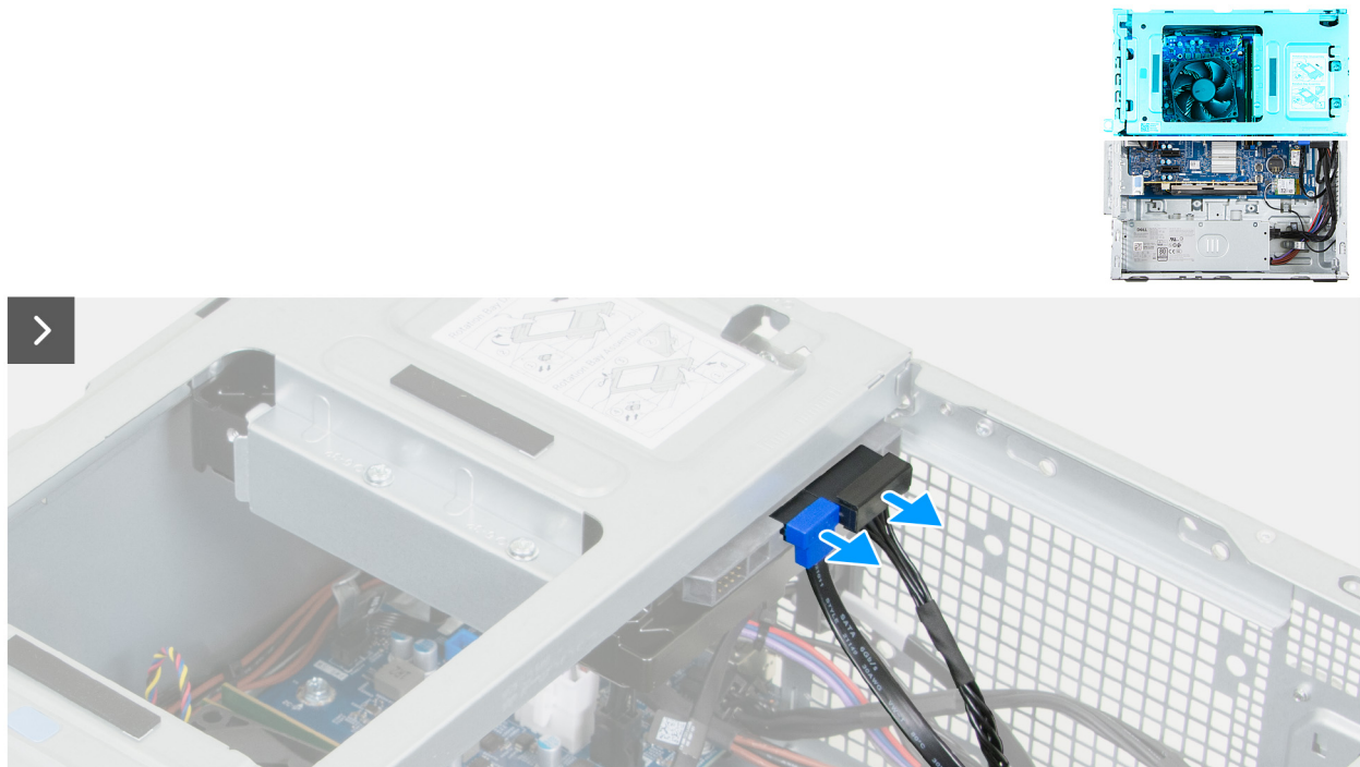
Figure 28. Removing the drive bay
