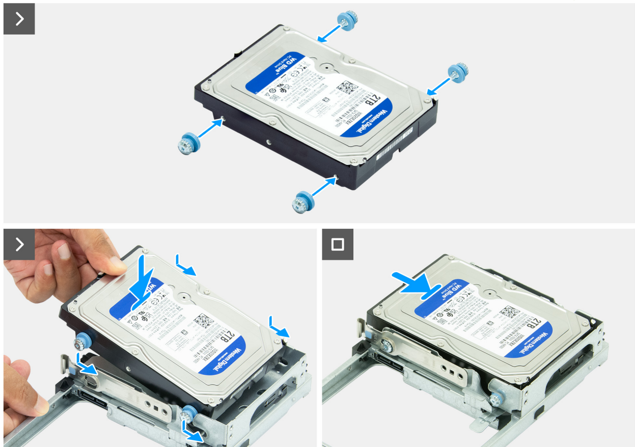
Figure 47. Installing the hard drive
