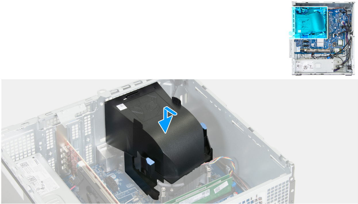
Figure 59. Image: Installing the fan shroud
