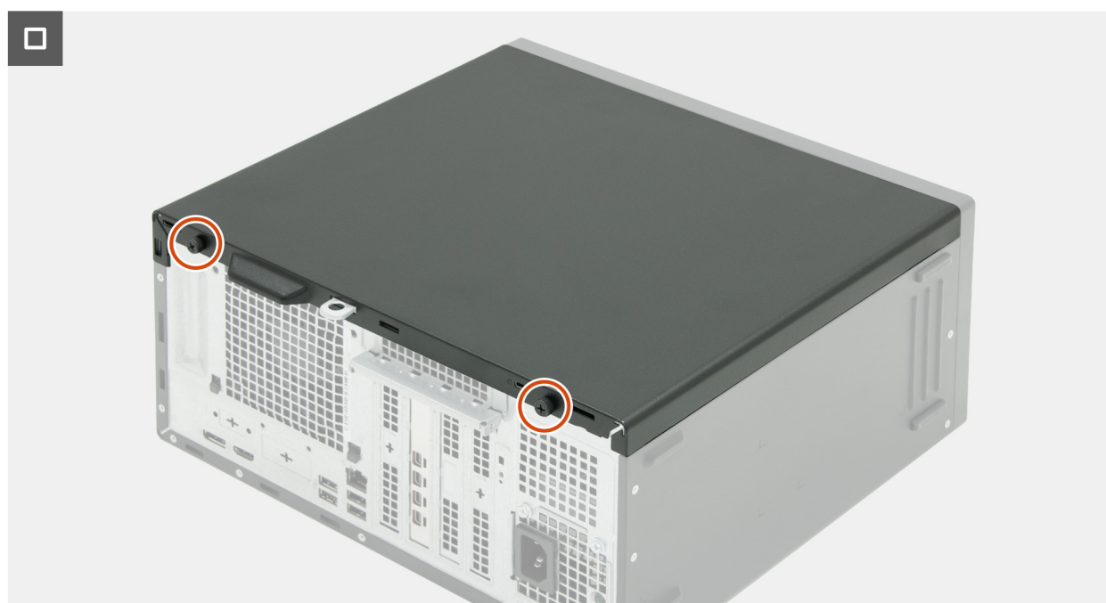
Figure 16. Installing the left-side cover
