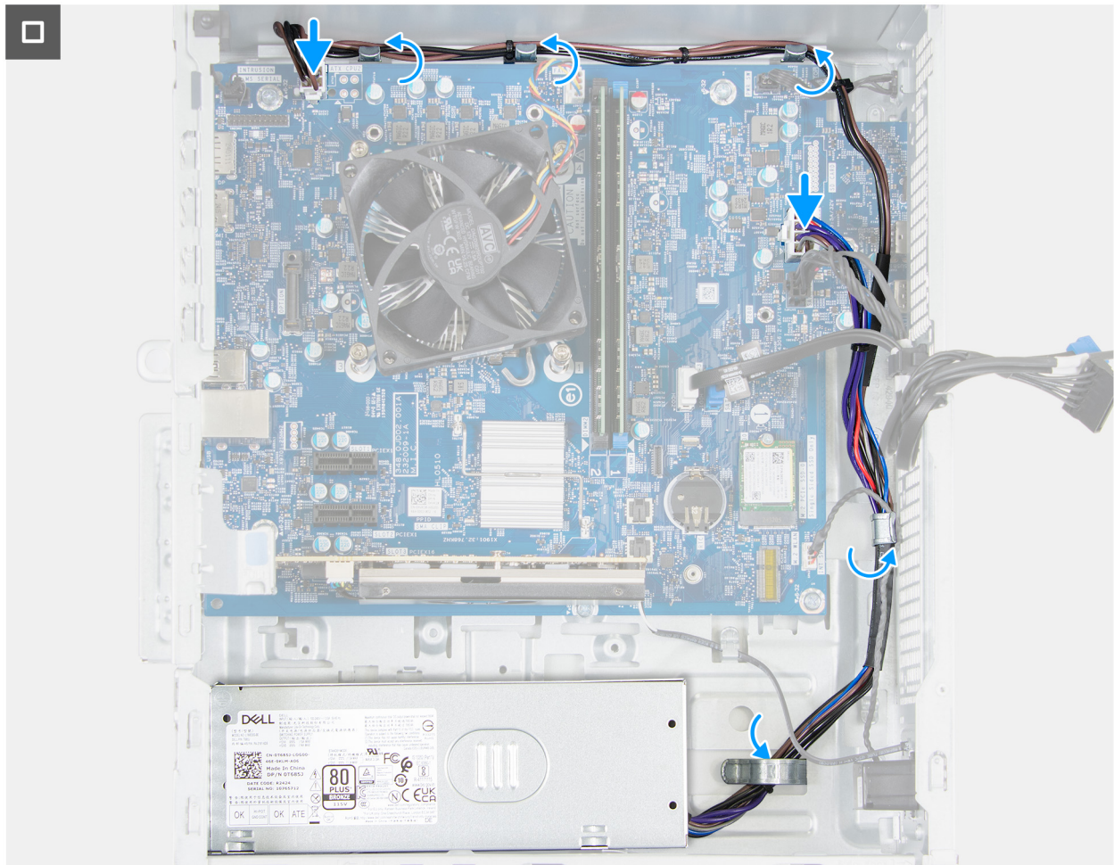
Figure 65. Installing the power-supply unit
