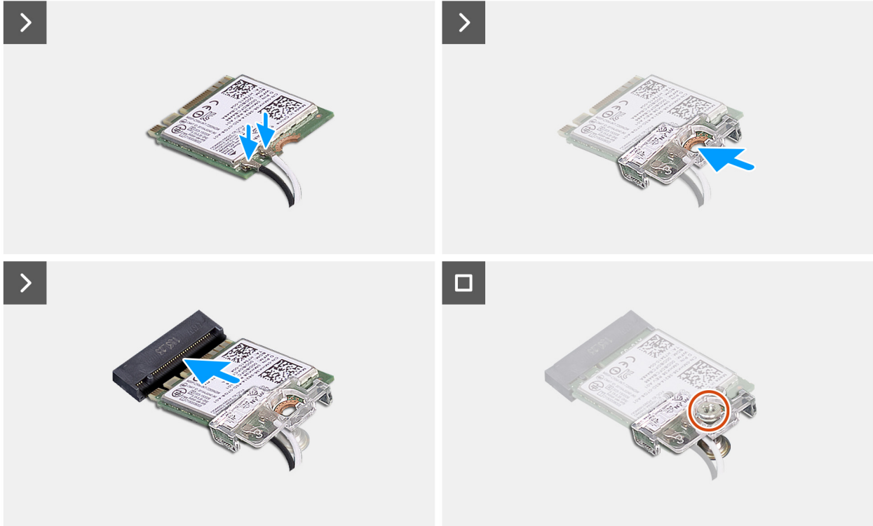
Figure 27. Installing the wireless card
