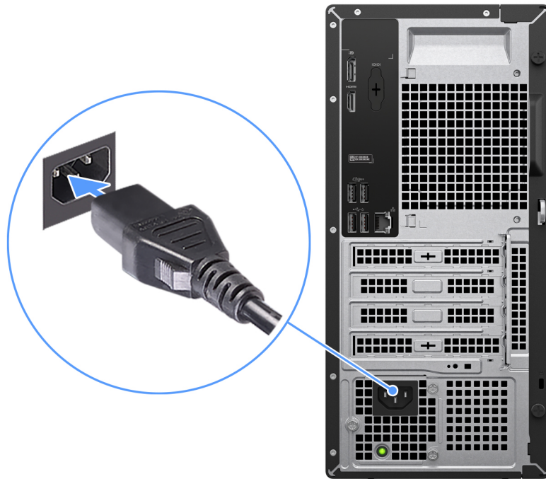
Figure 7. Connecting the power cable
