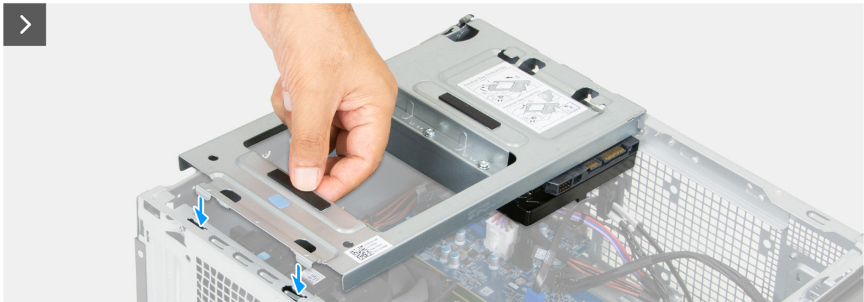
Figure 31. Installing the drive bay
