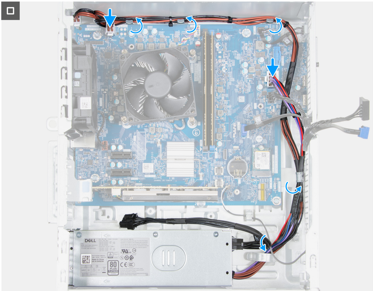
Figure 49. Installing the power-supply unit
