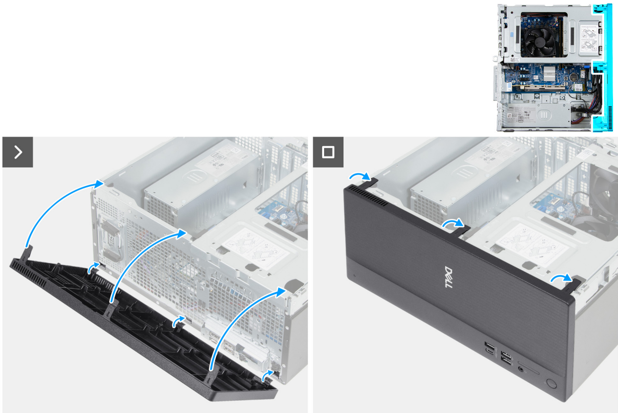
Figure 19. Installing the front cover
