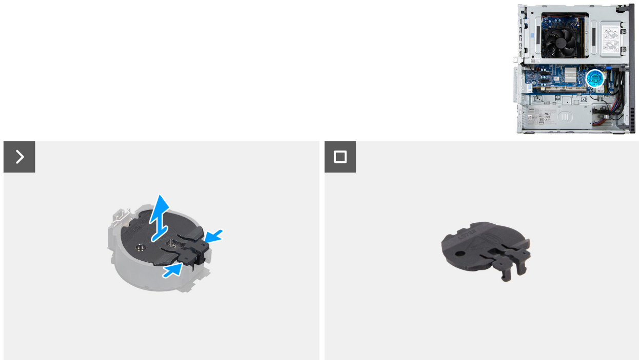
Figure 14. Removing the coin-cell battery cover
