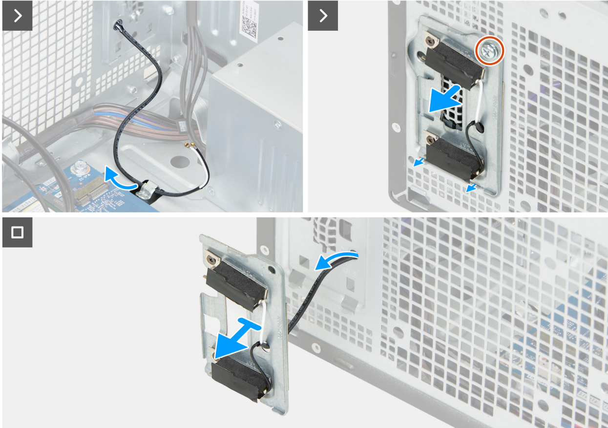
Figure 44. Removing the antenna modules
