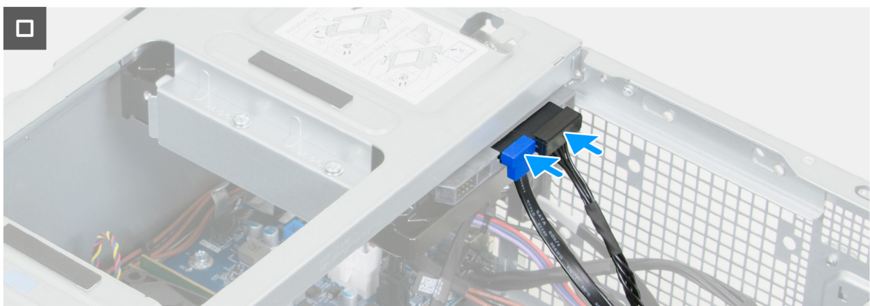
Figure 32. Installing the drive bay
