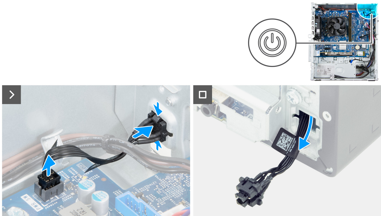
Figure 35. Removing the power button
