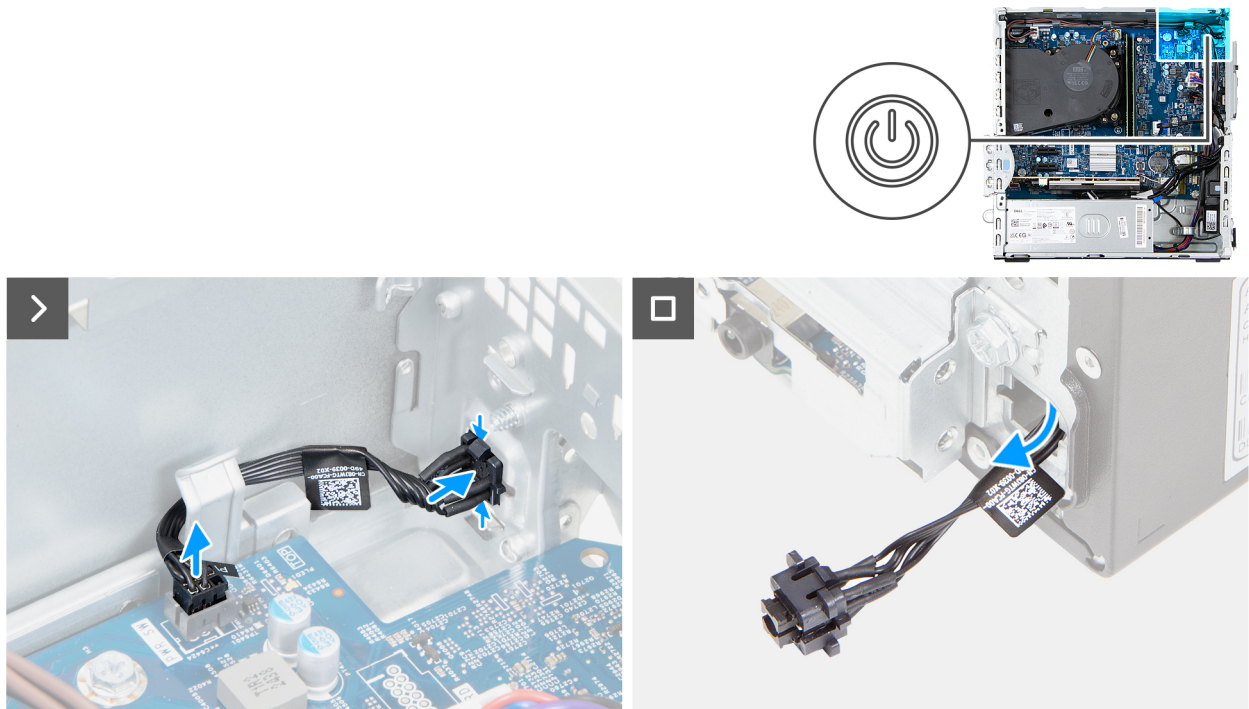
Figure 44. Removing the power button
