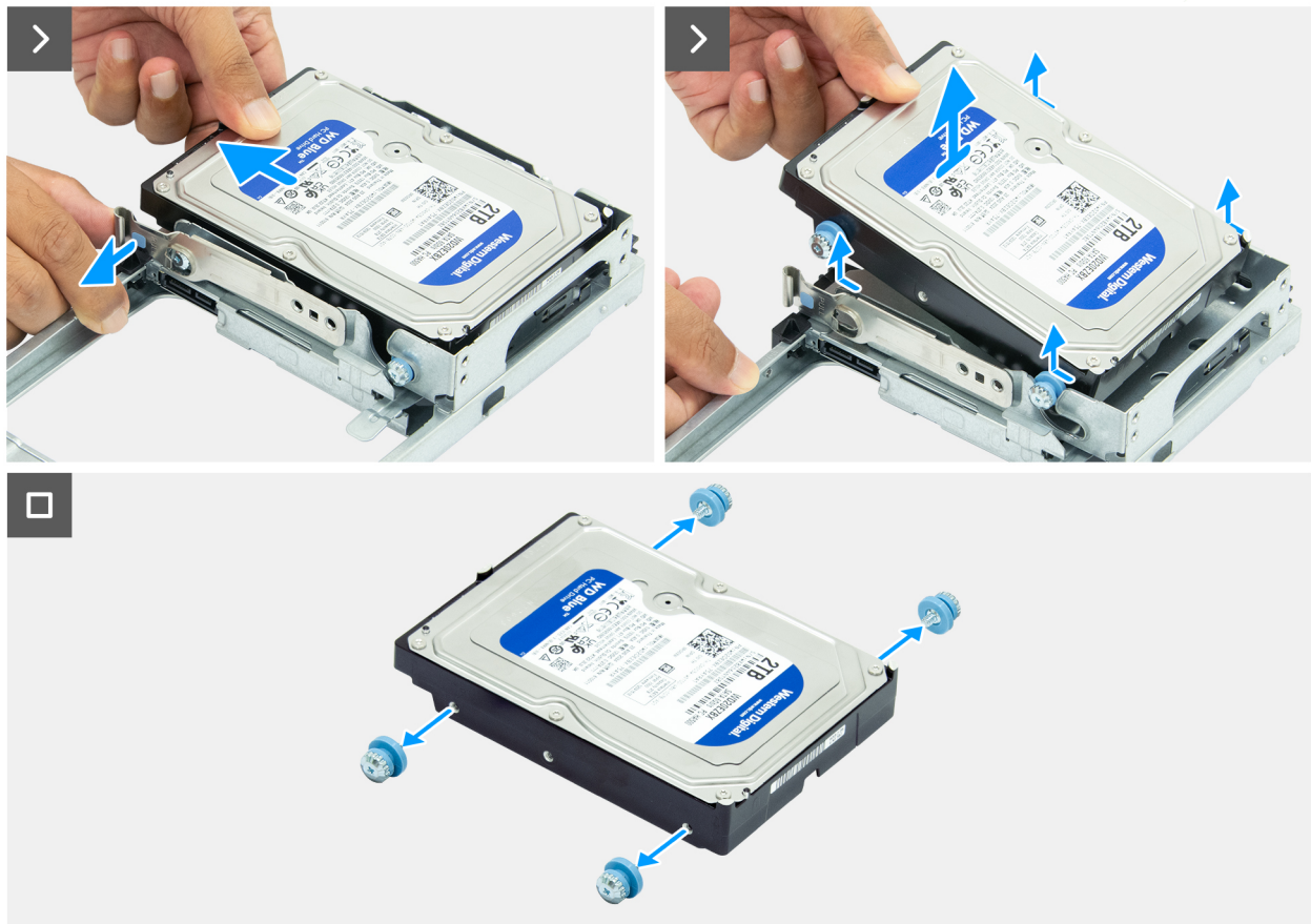
Figure 40. Removing the hard drive
