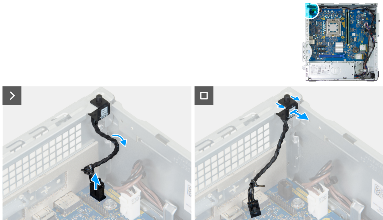
Figure 42. Removing the intrusion switch
