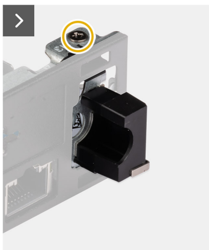
Figure 68. Installing the antenna module (white cable)
