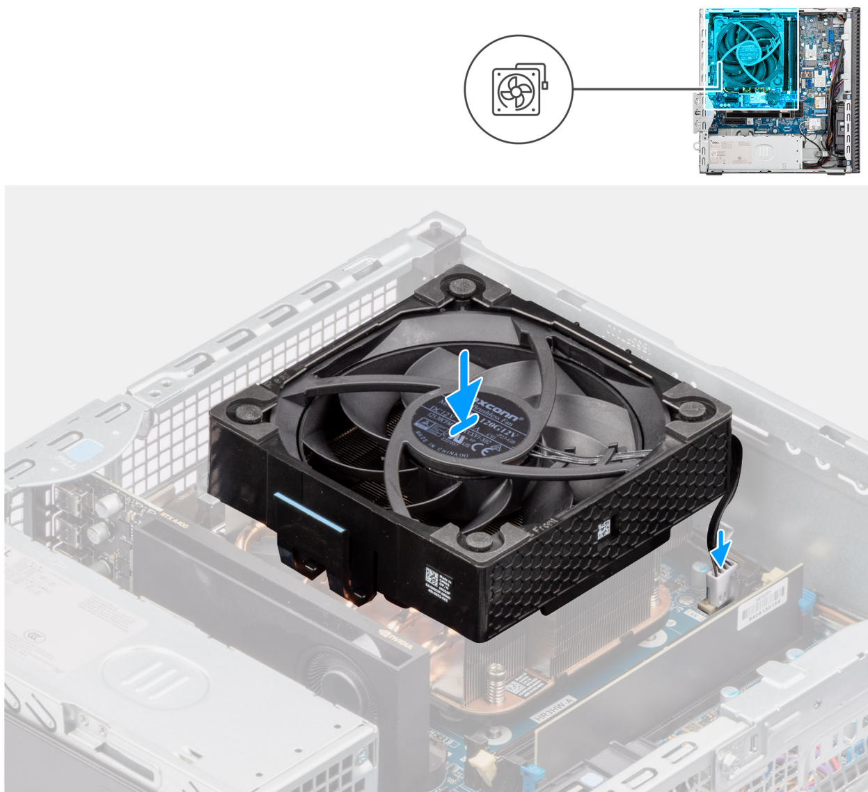
Figure 52. Installing the processor fan
