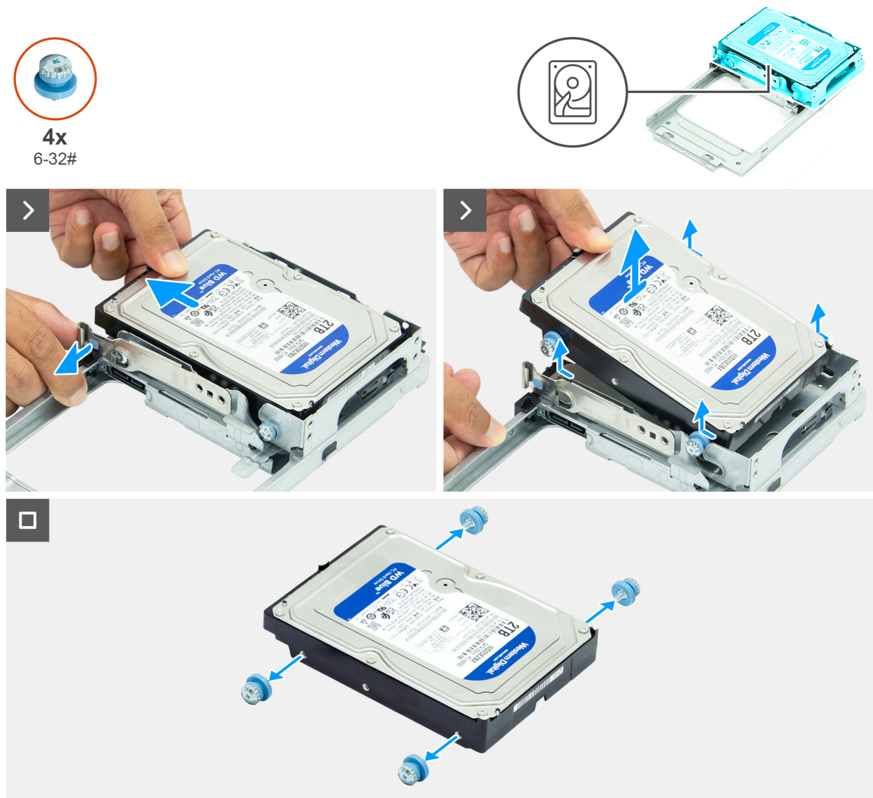
Figure 29. Removing the hard drive
