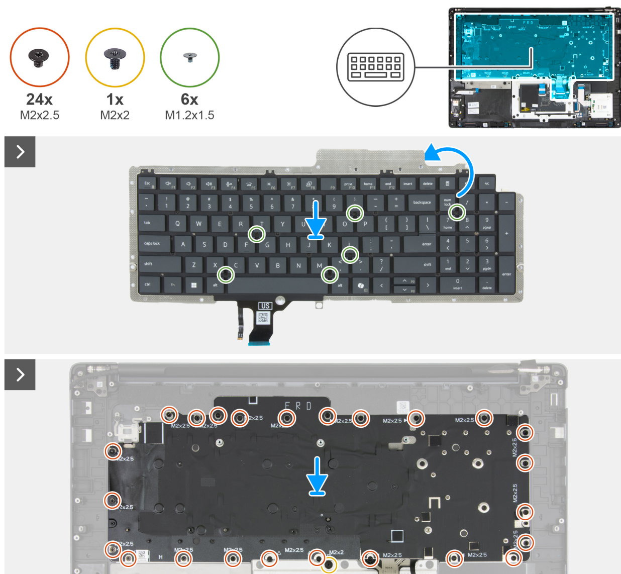
Figure 119. Installing the keyboard
