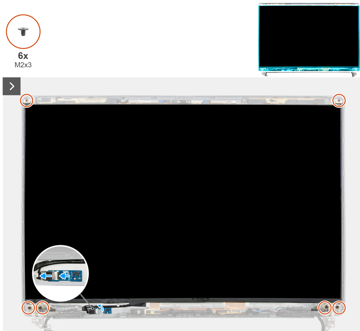
Figure 95. Removing the display panel
