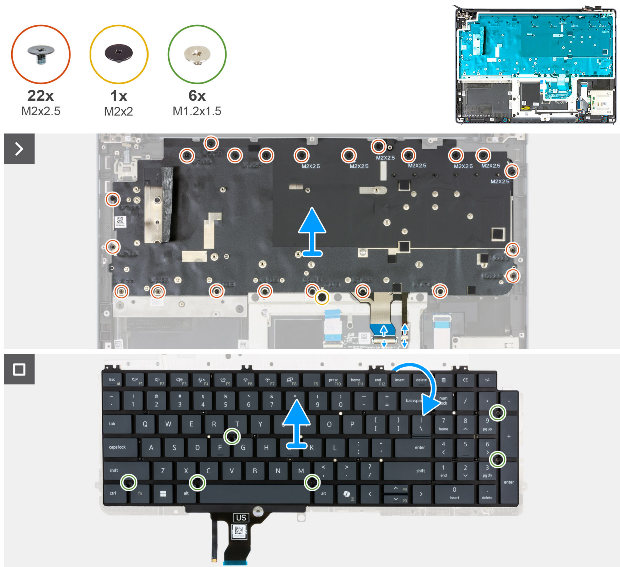
Figure 119. Removing the keyboard
