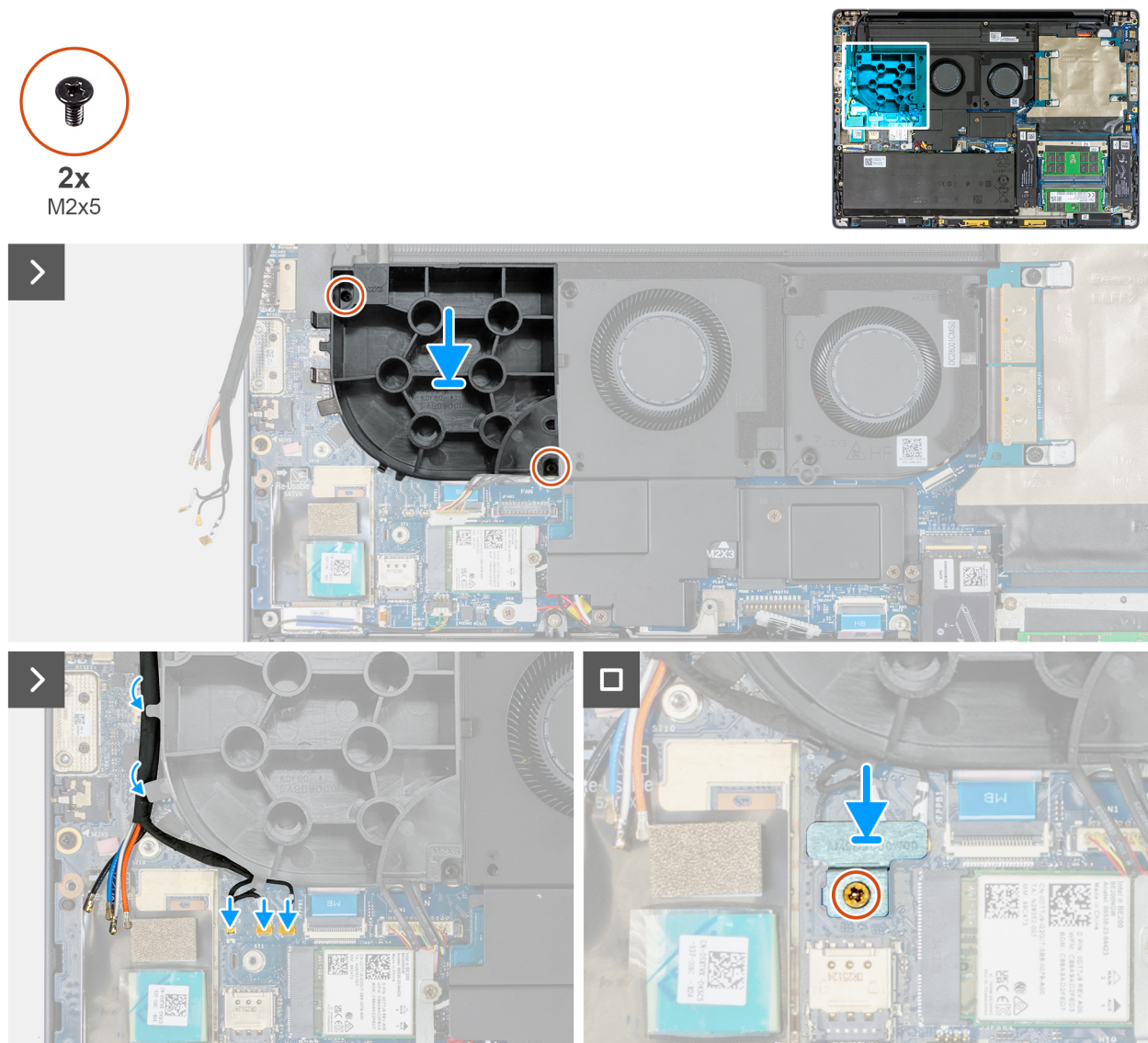
Figure 60. Installing the dummy fan
