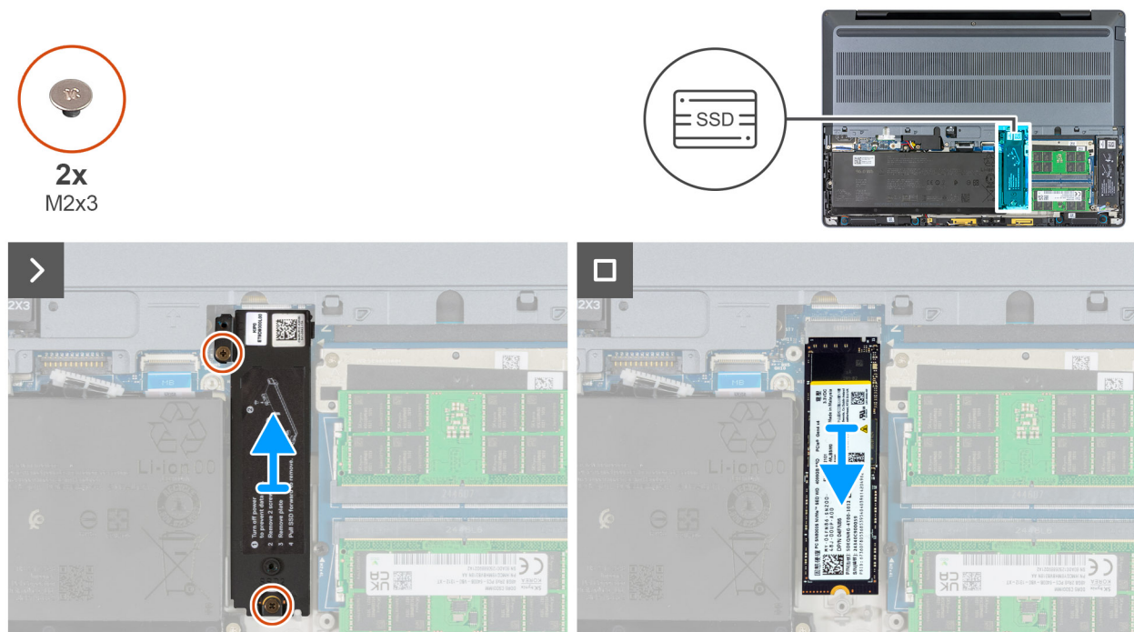
Figure 38. Removing the M.2 2280 SSD from slot 2 (SSD2)
