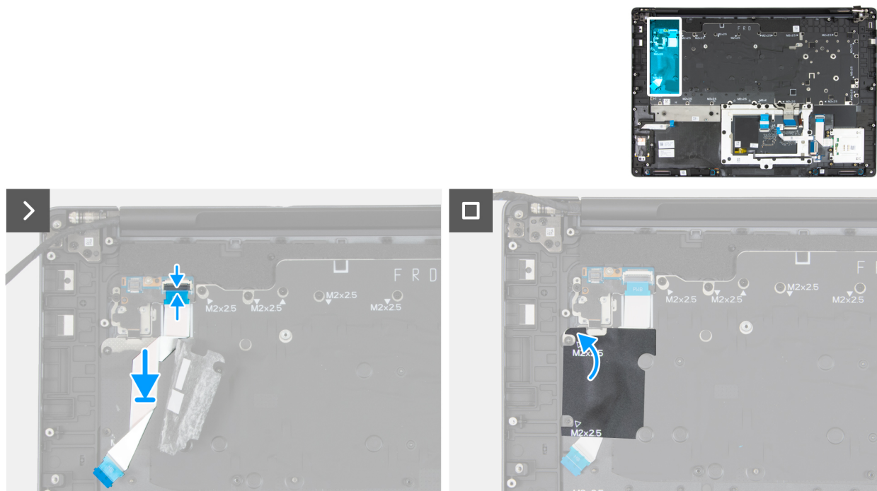
Figure 124. Installing the power button board cable
