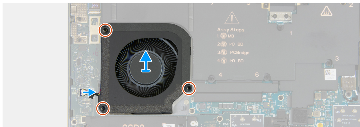
Figure 32. Removing the right fan
