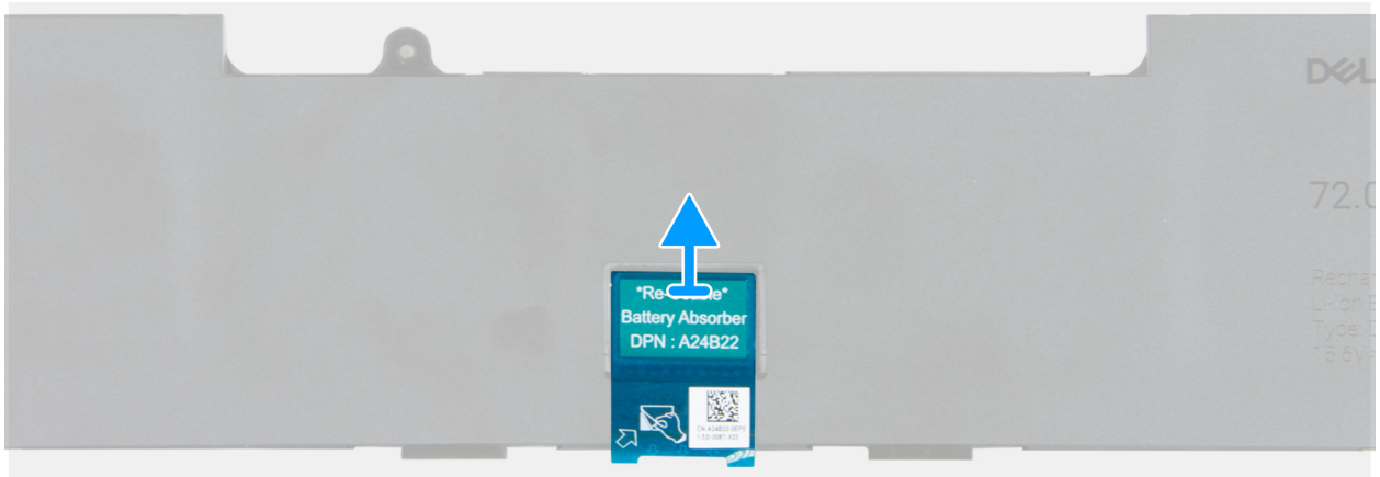
Figure 18. Removing the battery absorber
