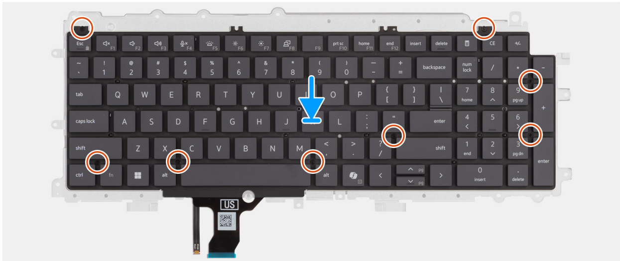
Figure 69. Installing the keyboard support plate
