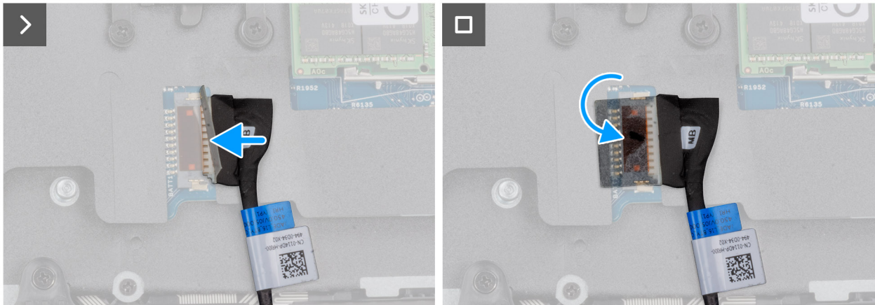
Figure 14. Connecting the battery cable
