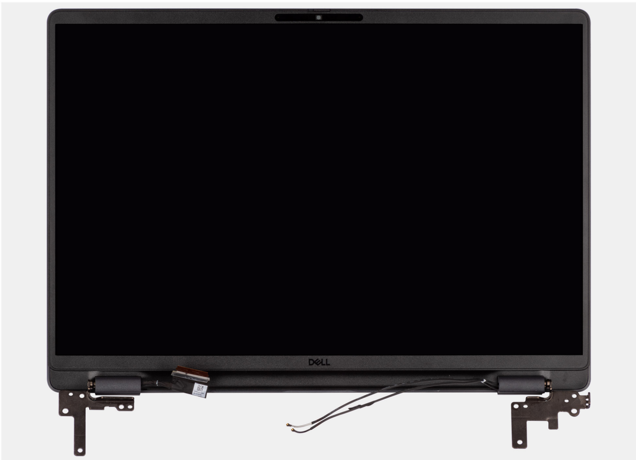
Figure 74. Removing the display assembly
