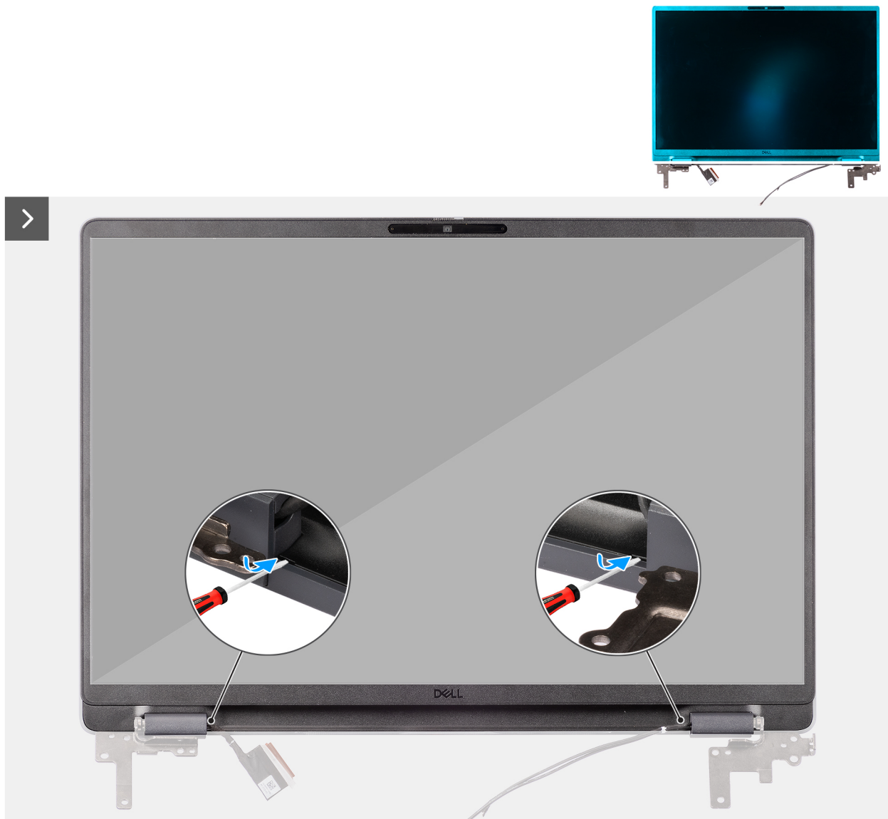
Figure 77. Removing the display bezel
