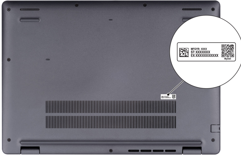
Figure 6. Service Tag/Express Service Code location
