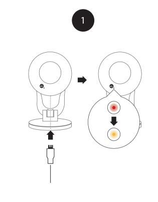
Plug the included USB Power Adapter into the back of the camera. Wait until the LED changes from red to blinking orange.
