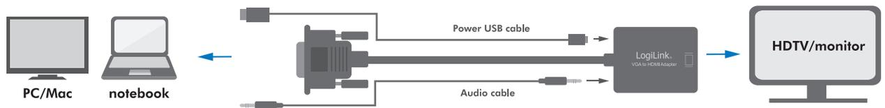
Ideal converter for VGA and Audio signals into HDMI signals
