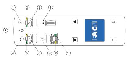
The ePDU front panel includes communication and monitoring ports. LED status indicators, and operation buttons. The ports and the associated LED indicators are described in the following table
