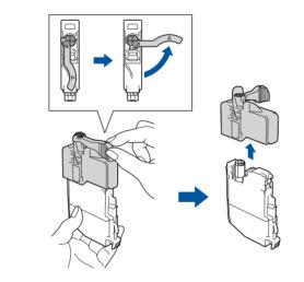
Quickly shake just the **black** ink cartridge horizontally 15 times as shown, before inserting it into the machine.
