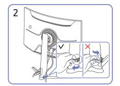
Pull the right side of the HOLDER-STAND CABLE to remove from the stand. The left side of the HOLDER-STAND CABLE can be damaged when pulled forcibly.
