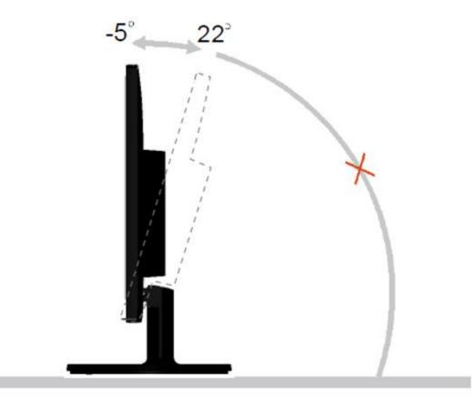
2> You are able to adjust the monitor's angle from -5° to 22 °.
