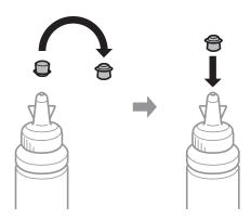
9. Close the cap onto the ink tank securely.
