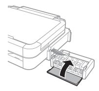
11. Hook the ink tank unit onto the printer.
