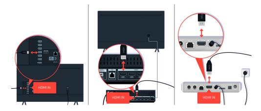
Check the antenna and HDMI cable connections.
