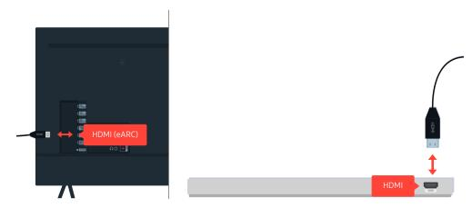
If no sound comes out of your Sound Bar, and if it is connected to the TV with an HDMI cable, check the HDMI (eARC) connector on the back of the TV.
