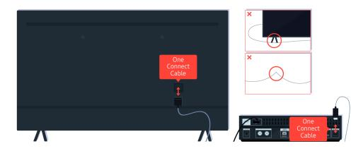
Disconnect and reconnect the One Connect cable between the TV and the One Connect (OC) Box. Make sure that the One Connect cable is not pinched or bent sharply.
