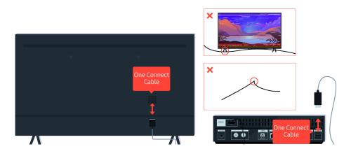
If the problem persists, and if your TV uses the One Connect Cable, disconnect and reconnect the One Connect Cable to the TV and the One Connect (OC) Box. Ensure that the One Connect Cable is not pinched or bent sharply.
