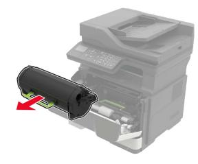
**3** Remove the used imaging unit.
