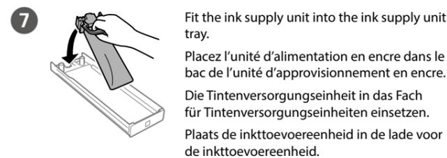
Fit the ink supply unit into the ink supply unit tray.
