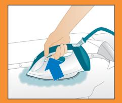
Press and hold the steam trigger for steam during ironing.
