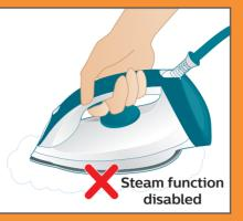
The steam function will be disabled automatically if descaling is not performed.
