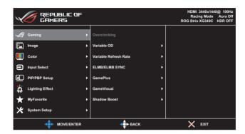
Overclocking: Allows to adjust the refresh rate.
